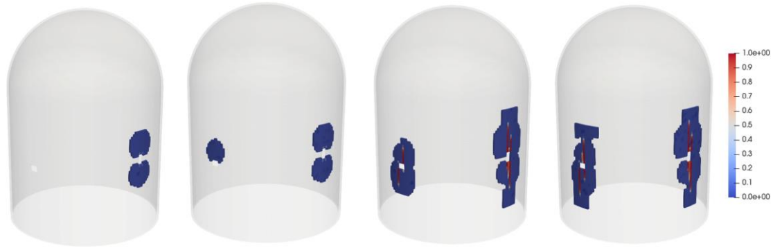
Figure 7. Application of the adaptive static condensation to a mockup of a containment building (VERCORS) [11]
