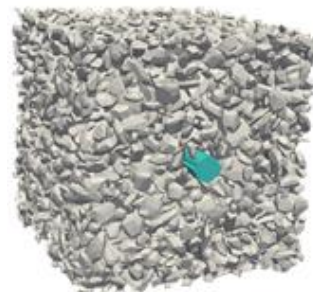
Figure 5. Mesoscopic representation of a concrete volumen including a steel bar
