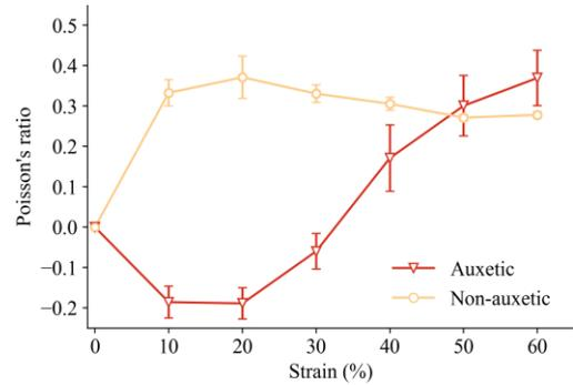
**Figure 3:** Poisson’s ratios for auxetic and non-auxetic lattice structures.
