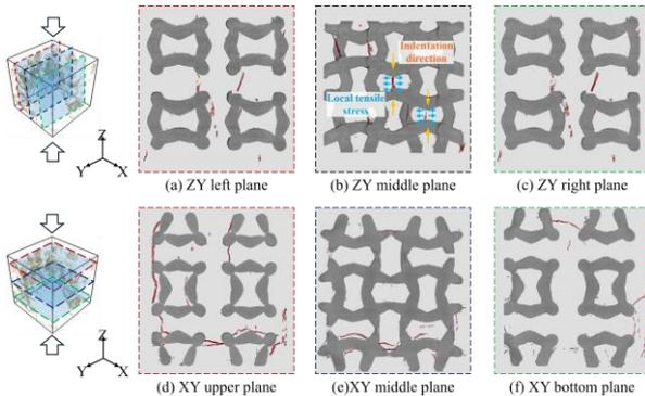
**Figure 7:** Microstructural damage for cementitious composites with auxetic lattice, where dark gray represents lattice and red represents cracks.
