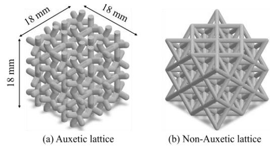
**Figure 1:** Geometry design of lattice structures.
