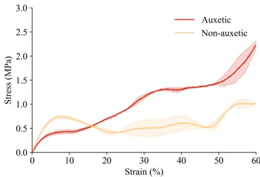
**Figure 2:** Compressive stress–strain curves of auxetic and non-auxetic lattice structures.
