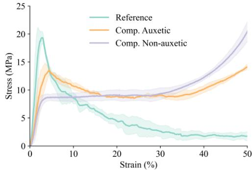
**Figure 4:** Compressive stress–strain curves of cementitious composites and reference mortar.
