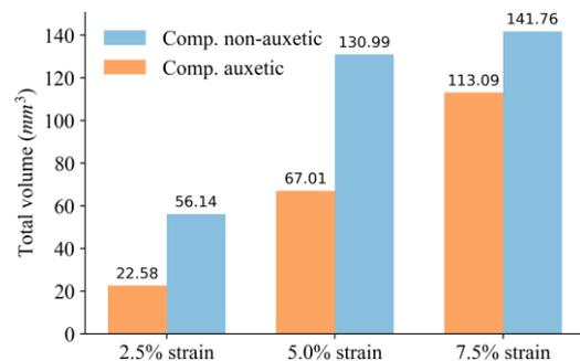
**Figure 6:** Crack volumes for cementitious composites with auxetic and non-auxetic lattice structures.
