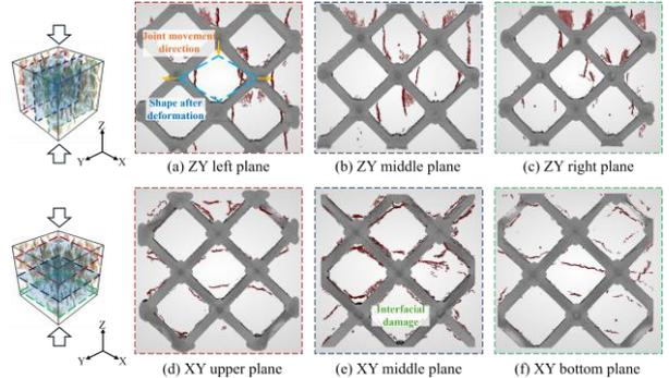
**Figure 8:** Microstructural damage for cementitious composites with non-auxetic lattice.
