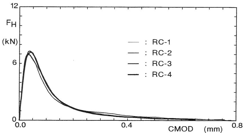
b) Concrete with aggregate from recycled concrete
