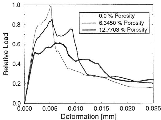
Fig.5. The effect of porosity on load-deformation behaviour.
