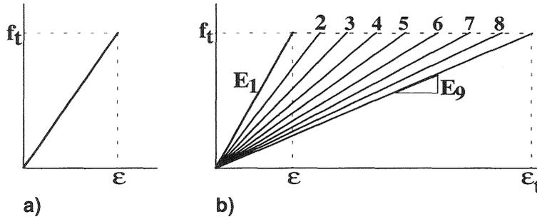
Fig.2. a) Stress-strain relation of lattice elements in linear elastic analysis, b) Calculation procedure in non-linear elastic analysis.
