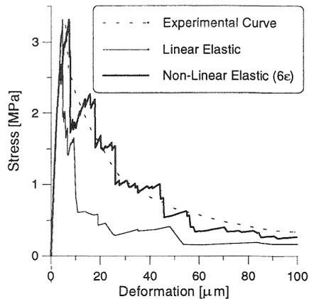
Fig 3. The effect of the fracture law on load-deformation response.
