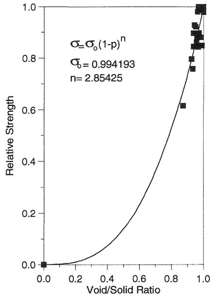
Fig.7. Comparison of numerically determined strengths and Power's law
