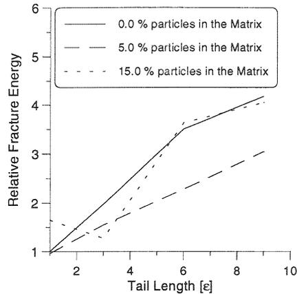
Fig 4. The effect of tail length in the fracture law and the particle ratio on the fracture energy
