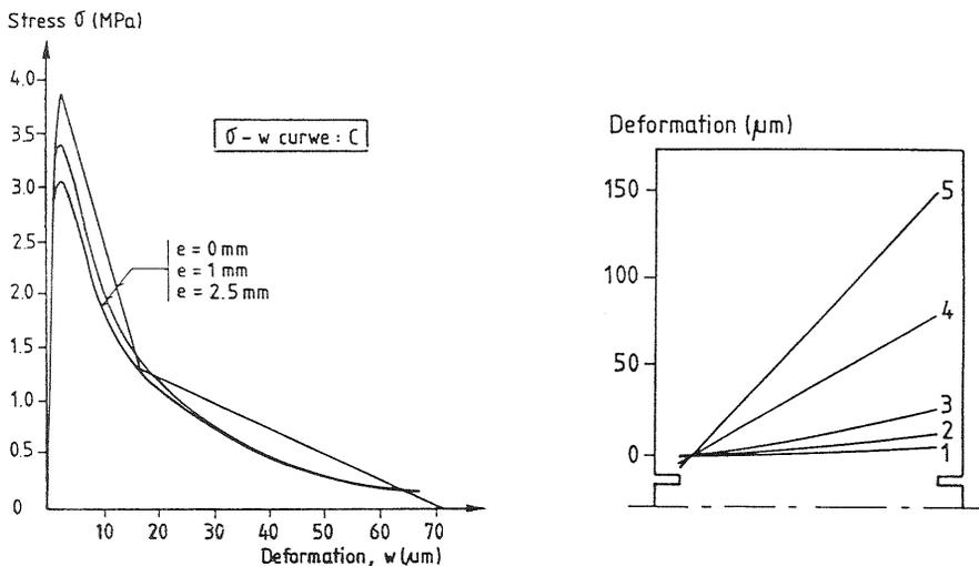
Fig. 5 Influence of eccentricity on the stress-deformation curve and deformation distribution across the fracture cross-section.
