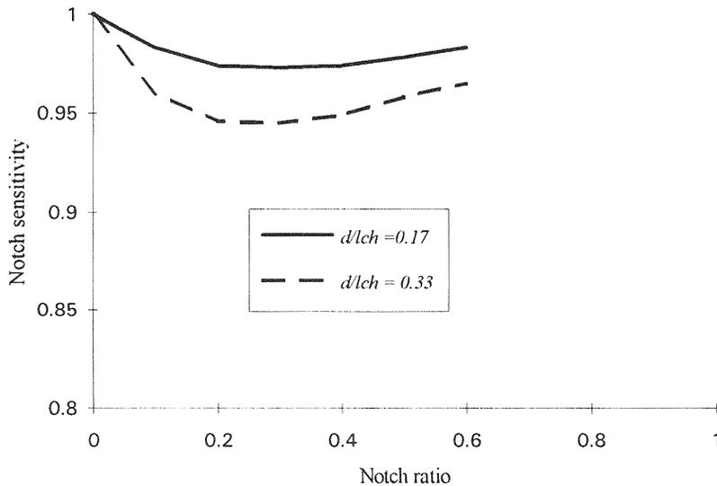
Fig. 3 Notch sensitivity of tensile strength predicted by FCM.
