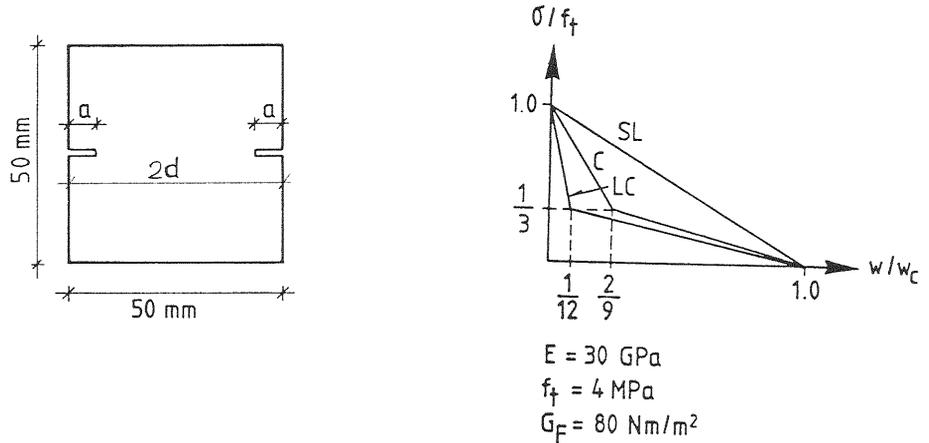
Fig. 1 Dimensions of specimen and stress-deformation curves.
