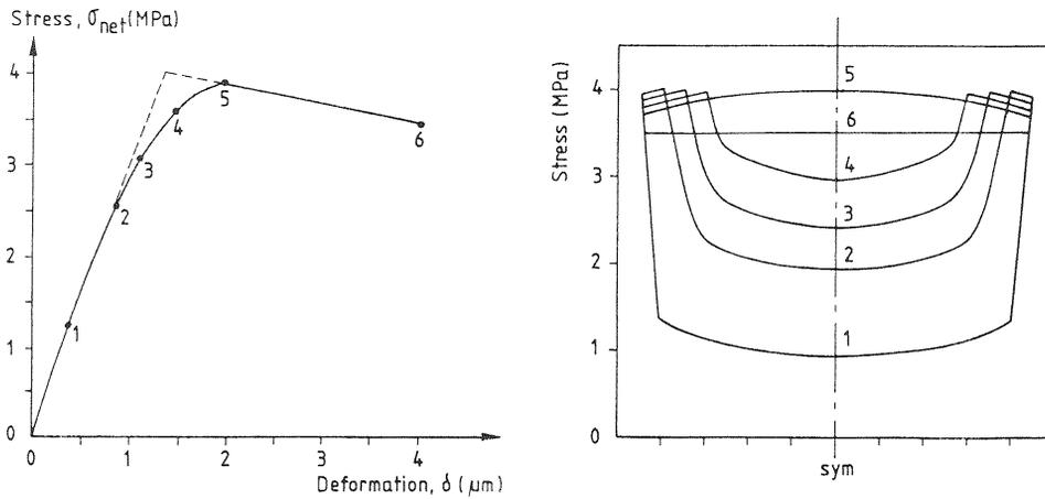
Fig. 2 Simulated (solid line) and true (dash line) stress-deformation curves and stress distributions across the fracture cross-section.
