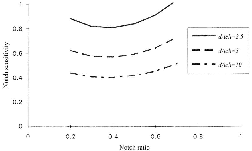
Fig. 4 Notch sensitivity of tensile strength predicted by LEFM.
