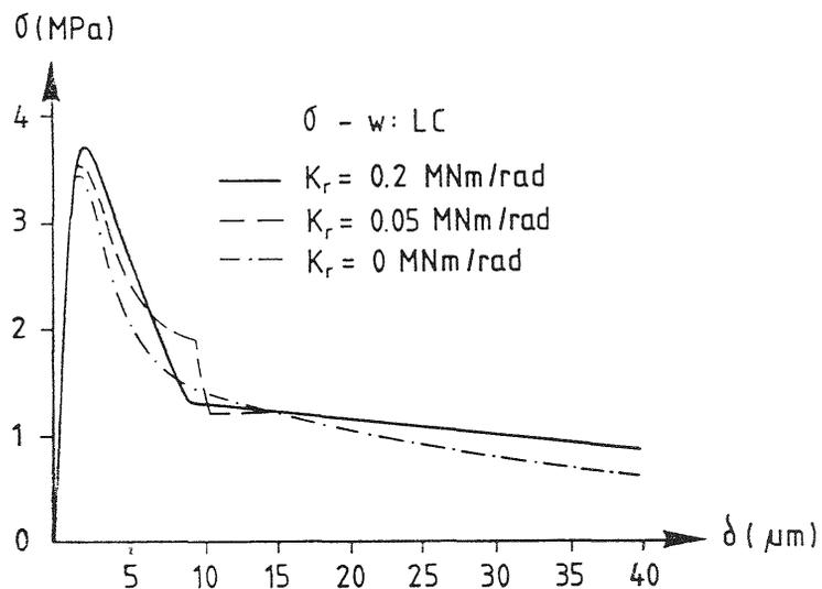
Fig. 6 Effect of rotational stiffness on tensile tests.
