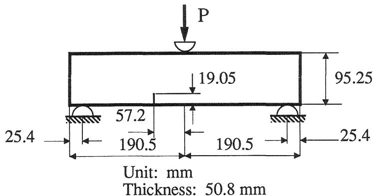
Fig. 1. SEN three point bend concrete specimen
