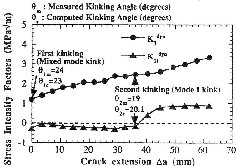
Fig. 8.  $K_I^{dyn}$  and  $K_{II}^{dyn}$  variations with crack extension
