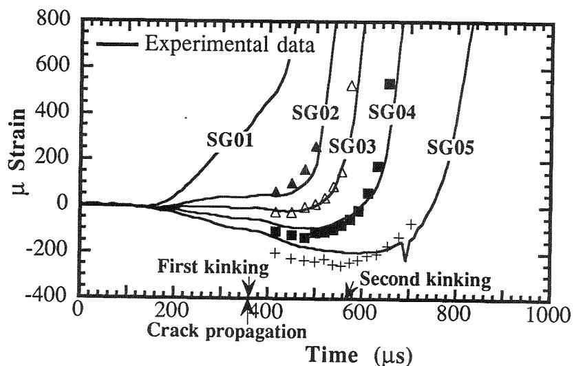
Fig. 4. Measured and computed average strain history
