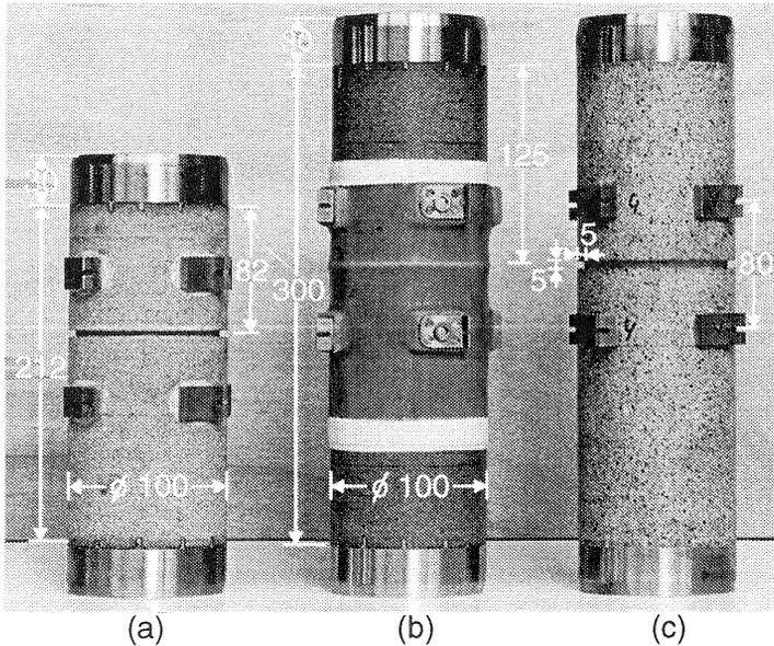
Fig. 3 Dimensions of an open sandstone specimen (a), a closed sandstone specimen (b) and a mortar specimen (c)
