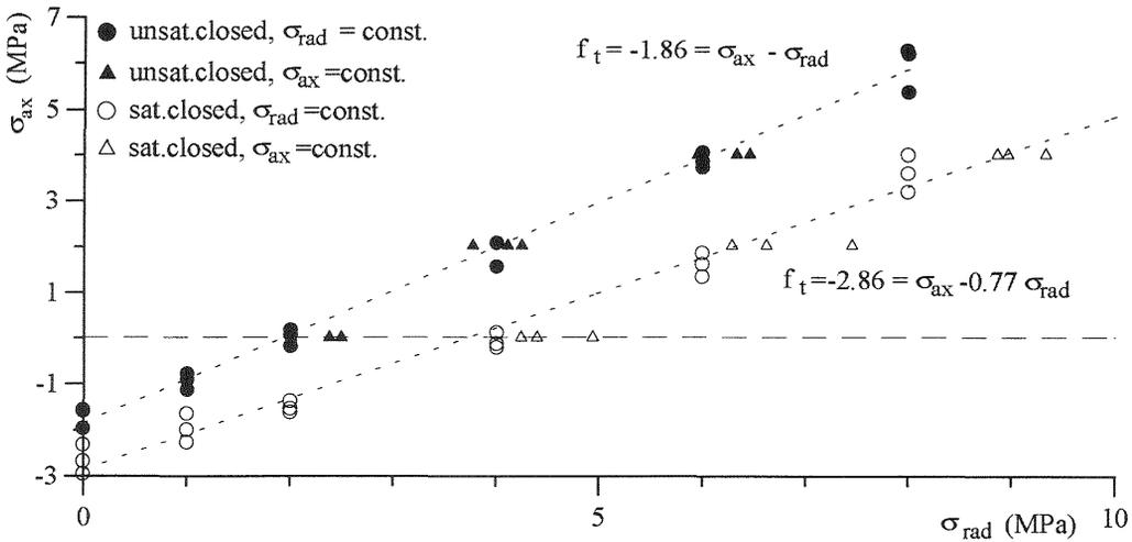
Fig. 5 Failure stresses for the mortar specimens
