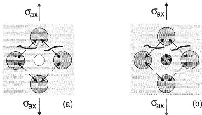
Fig. 7 Reaction forces under a global tensile stress for an unsaturated (a) and a saturated (b) porous material
