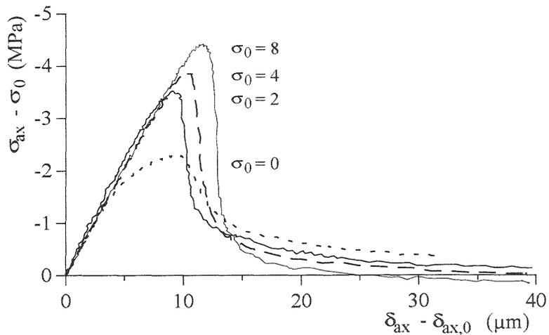
Fig. 4 Response curves of the saturated mortar specimens for different hydrostatic pre-loading stresses
