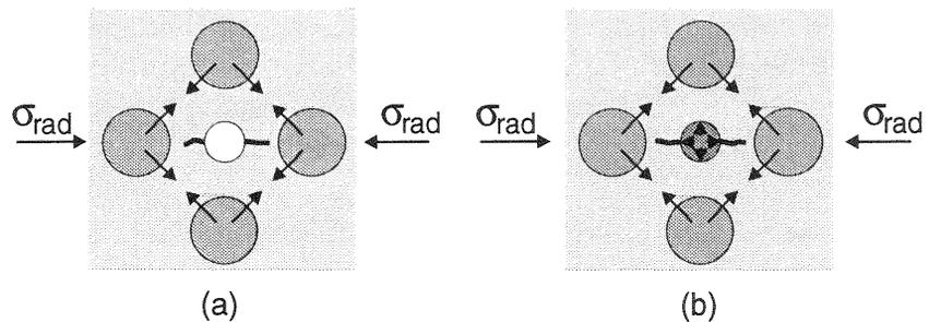
Fig. 8 Reaction forces under a global radial compressive stress for an unsaturated (a) and a saturated (b) porous material. The global radial stress is in the plane perpendicular to the drawing
