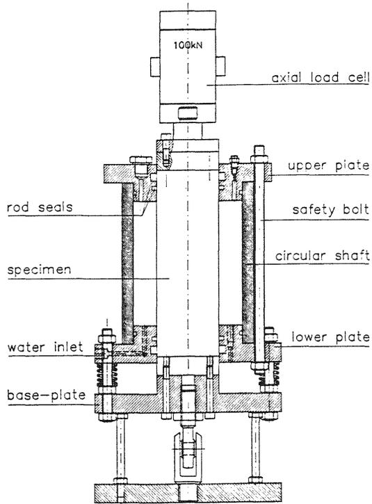
Fig. 1 The hydraulic cell
