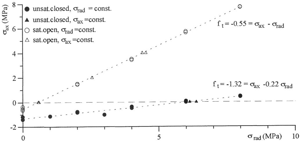
Fig. 6 Failure stresses for the Felsler sandstone specimens
