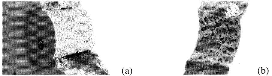
Fig. 7. Detailed observations of fracture in the IZ. In Fig. (a) a detail is given from the fracture surface of the sandstone aggregate and (b) shows the surface of the matrix. In the experiment a mortar with w/c ratio of 0.4 was used. Note the large pores in figure (b).
