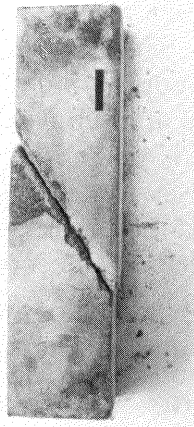
Fig. 6. Failure of specimen with weak layer: mater. B, 5 mm, 55°
