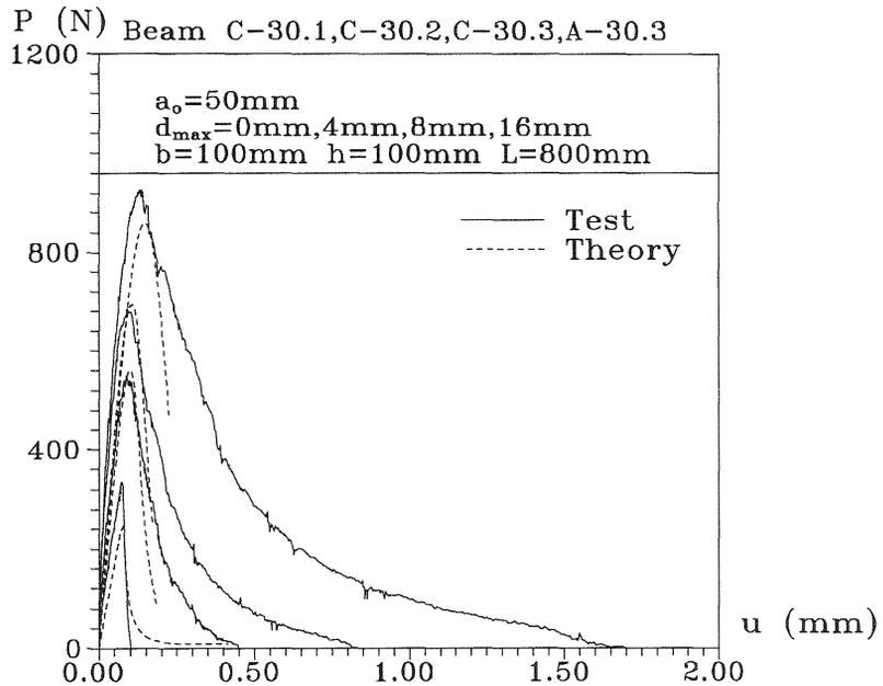
Fig. 6. Variation of aggregate size
