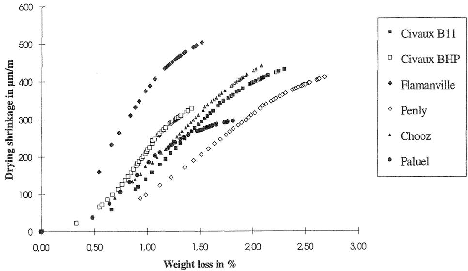
Fig. 1. Drying shrinkage vs weight loss for 6 French nuclear containment
