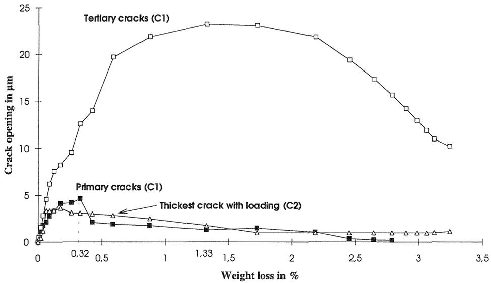
Fig. 5. Crack opening function of the weight loss in the two cases tested
