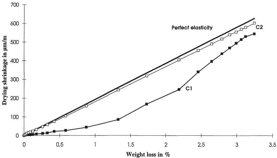
Fig. 6. Drying shrinkage as a function of the weight loss; comparison between experimental results and simulations C1 and C2
