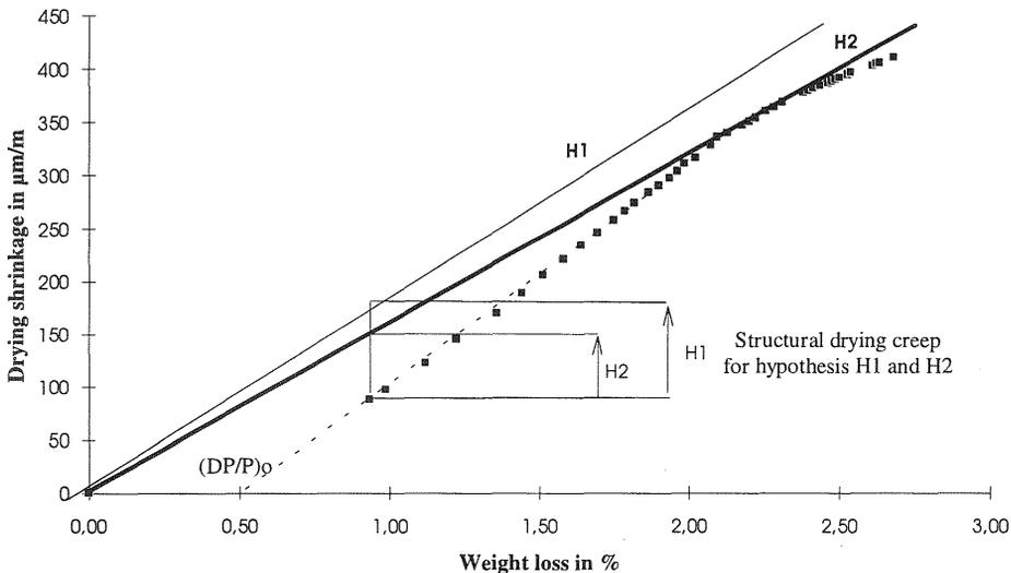
Fig. 2. Modelling of Penly's concrete according to hypotheses H1 and H2
