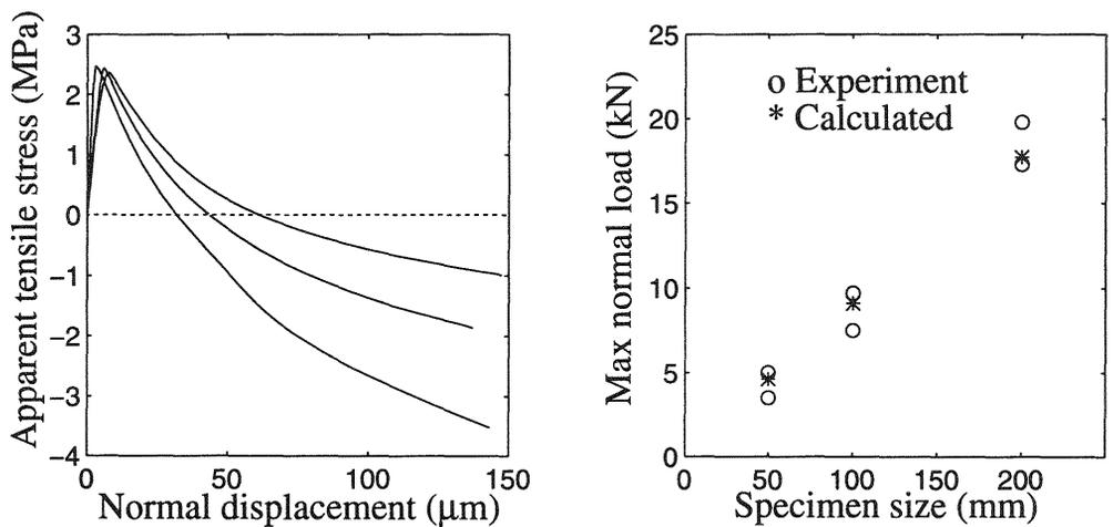
Fig. 3. Apparent tensile stress versus normal displacement and the maximum normal load as a function of specimen size
