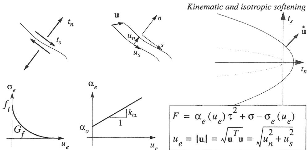
Fig. 1. Constitutive model of a fictitious crack under mixed mode conditions using Inner Softening Bands (ISB)
