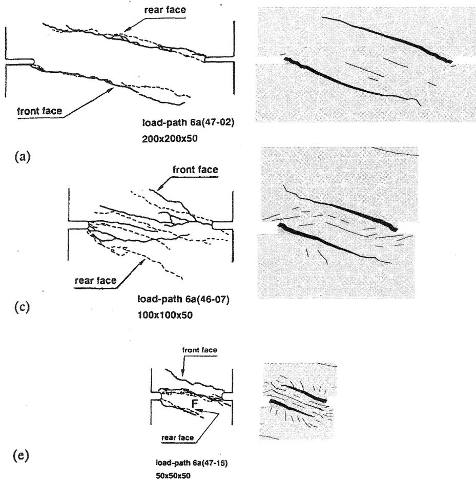
Fig. 4. To the left experimentally observed crack pattern for loadpath 6a, Nooru-Mohamed (1992). To the right calculated crack patterns at  $150\ \mu\text{m}$
