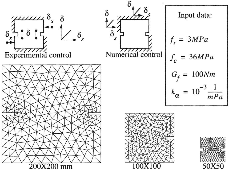
Fig. 2. FEM analysis of mixed-mode fracture test of three different sizes
