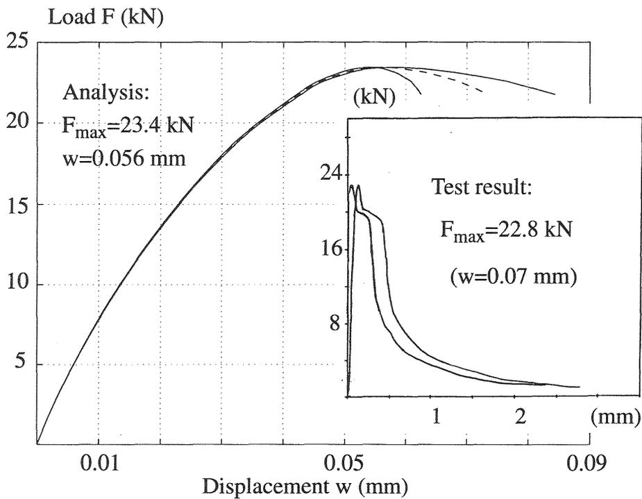
Fig. 7. Load displacement curve from the analysis together with experimental data from Ohlsson and Ghasemlou (1993)
