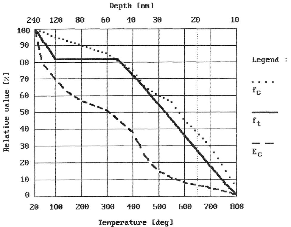
Fig.1 Degradation of concrete properties with temperature/depth (after Kordina and Meyer-Ottens, 1981)
