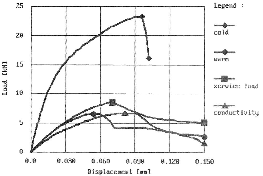
Fig.4 Load-displacement diagrams for an embedment depth 50 mm
