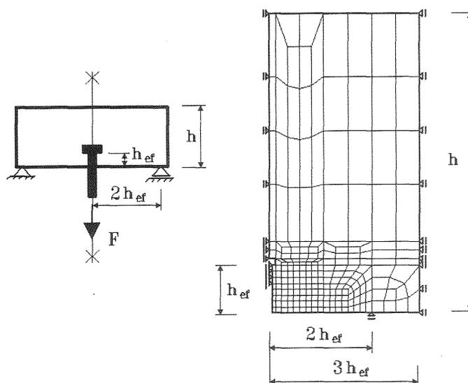
Fig.2 Scheme of the analytical model and finite element mesh
