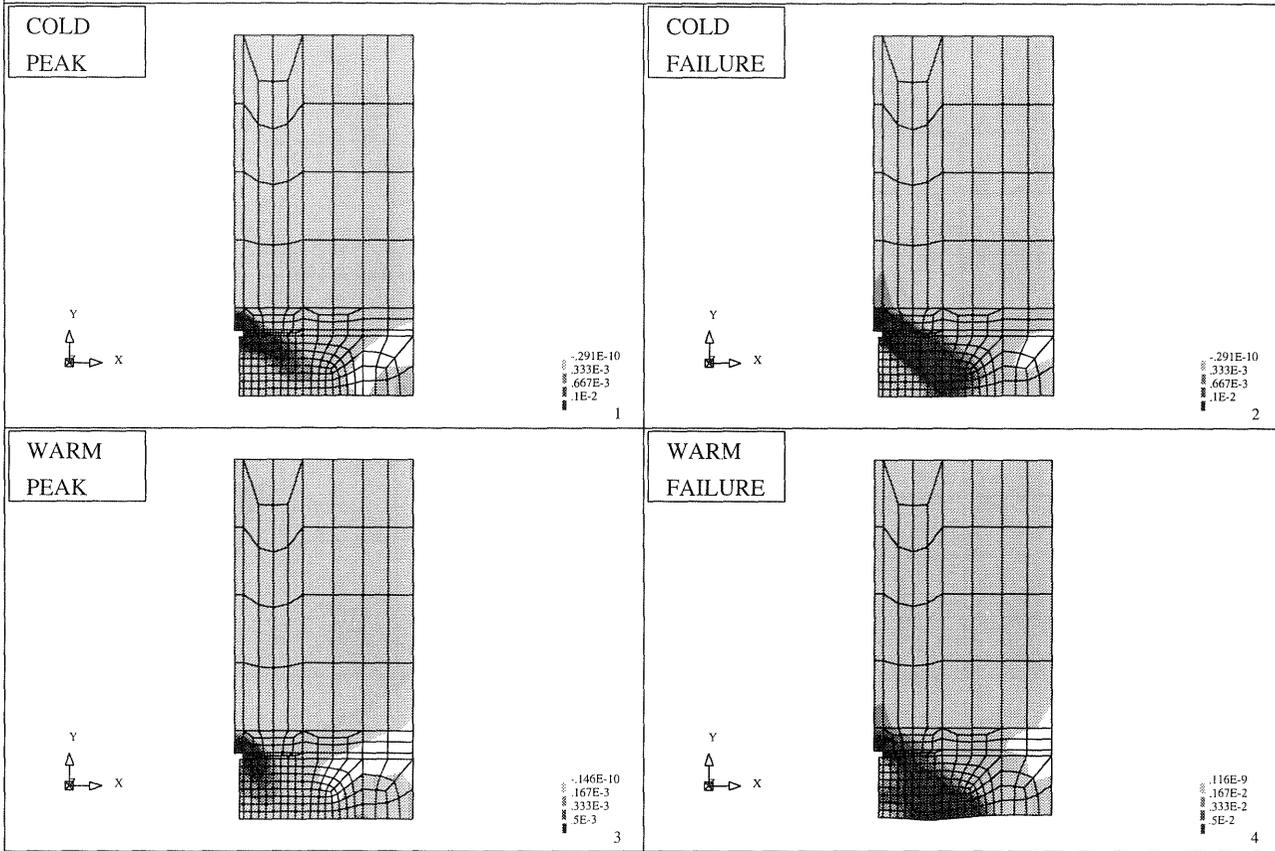
Fig.5 Distribution of principal tensile strains at peak load and at termination of the analysis, embedment depth 50 mm
