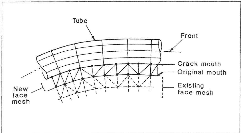
Figure 2: Crack face Delauney meshing
