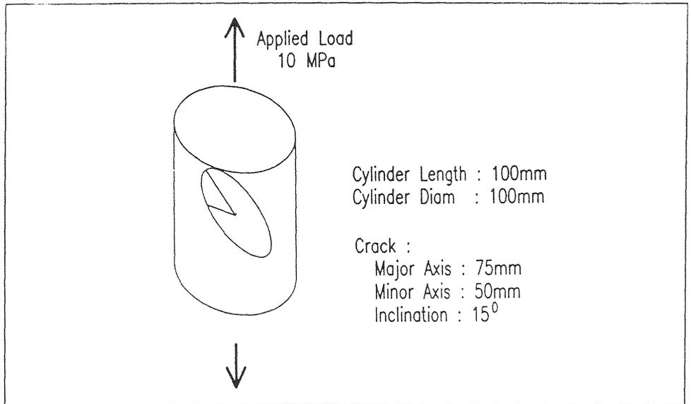
Figure 3: Inclined elliptical crack in a cylinder
