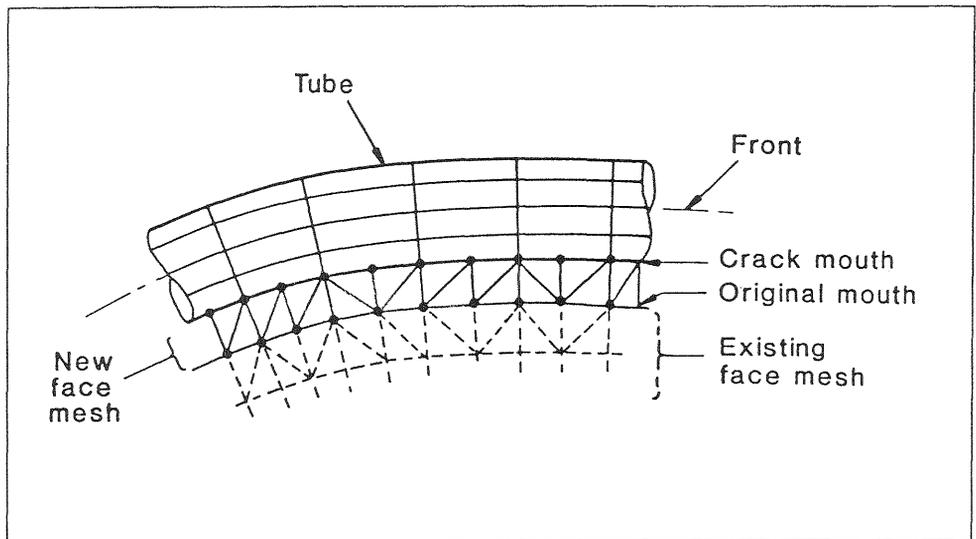
Figure 2: Crack face Delauney meshing
