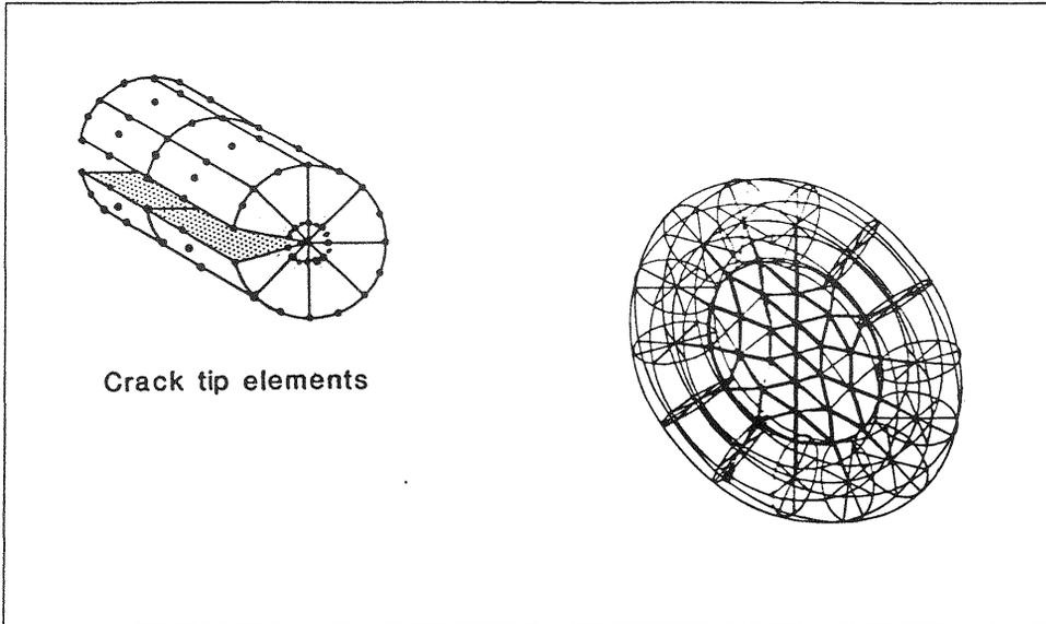
Figure 1: Crack tip elements - 'fracture tube'
