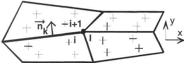
Fig. 1. Computation of the mesh indicator (node I)
