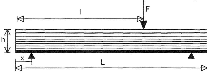
Fig. 2. Impact on beam (Geometry)
