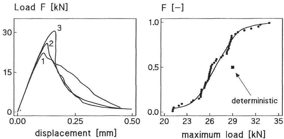
Fig. 6 (a) Load-displacement diagram. (b) Cumulative distribution of maximum load.
