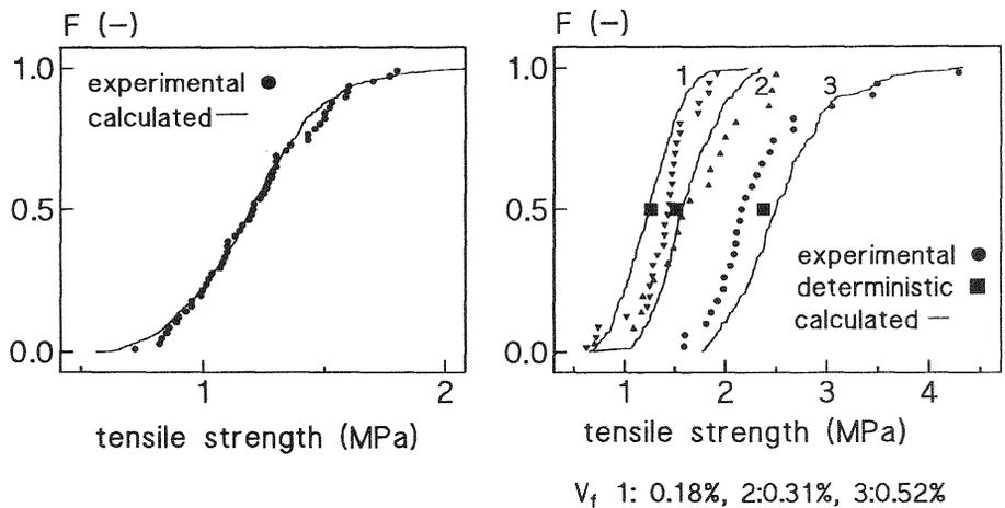
Fig. 3 (a) Cumulative distribution of tensile strength of polymer modified cement mortar.
