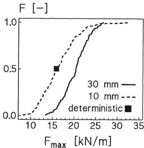
Fig. 4 Cumulative distribution of maximum load for two widths of beam in three point bending. Deterministic versus stochastic results.
