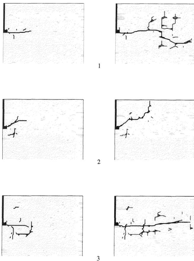
Fig. 7 Crack pattern at maximum load (a) and at final loading (b).
