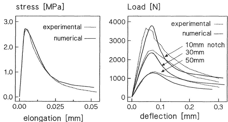
Fig. 1. Load-displacement curve for tensile test. Load-deflection curve for bending test for three notch depths.
