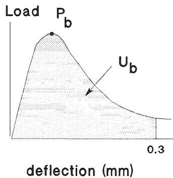
Fig. 2 Definition of structural response variables  $P_t$  and  $U_t$  for tensile test,  $P_b$  and  $U_b$  for bending test.
