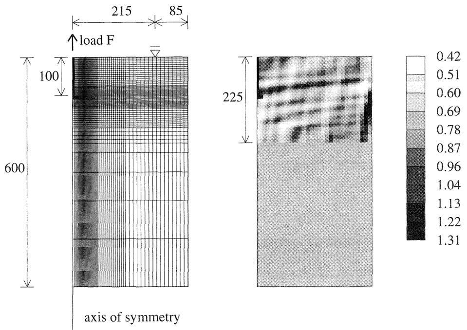
Fig. 5 Pull-out of an anchor bolt. Finite element and stochastic element model.
