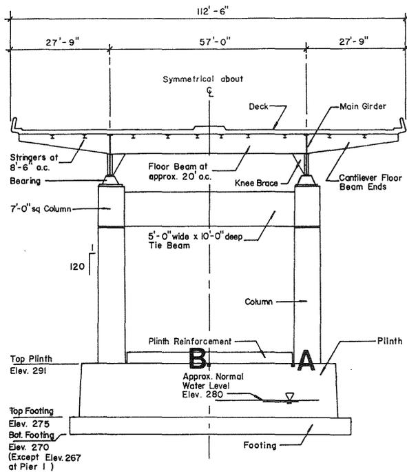
Fig. 5. Configuration of typical pier showing plinth reinforcement and initiation points for cracking. After Wiss87.
