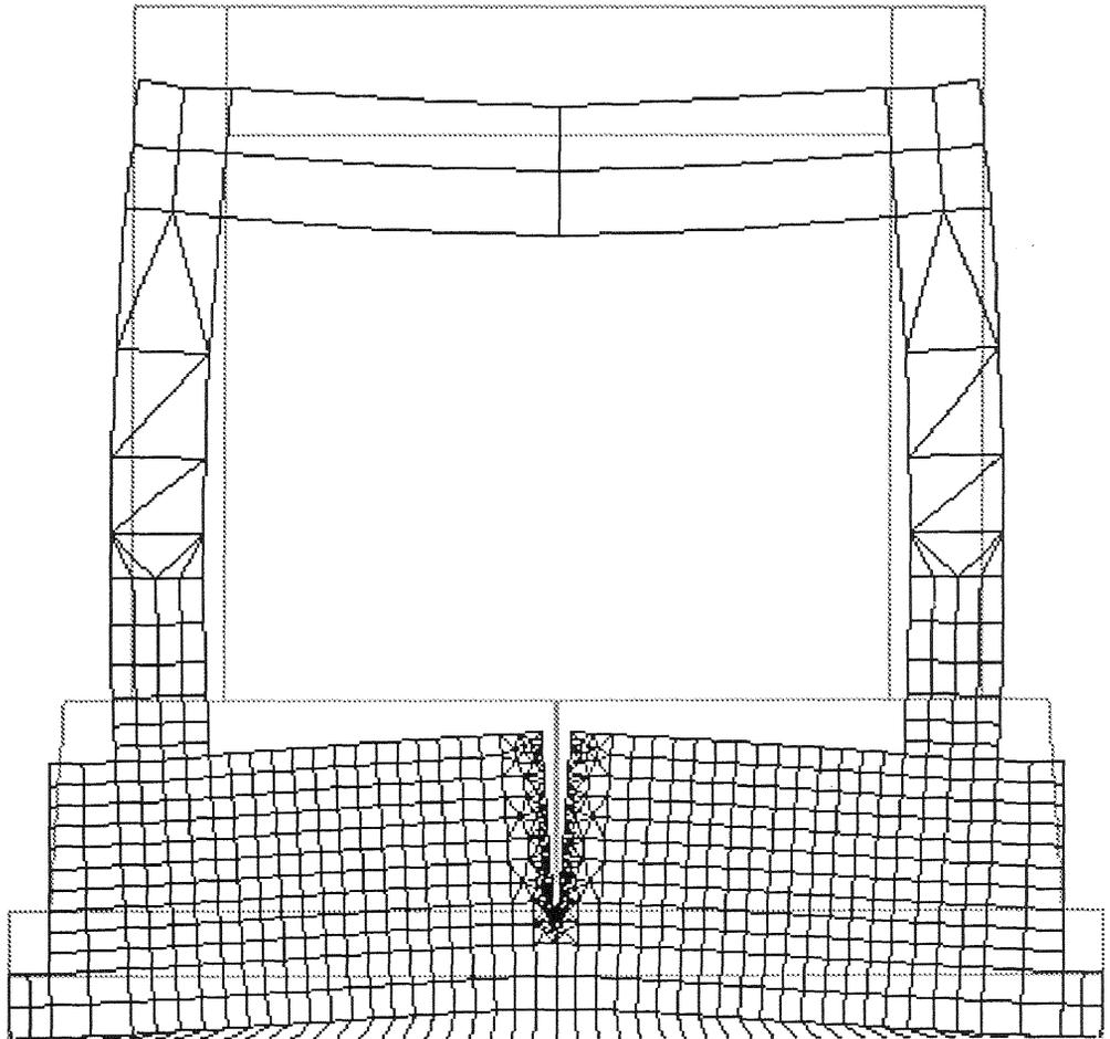
Fig. 9. Final deformed finite element mesh after fourteen 1 ft (0.30 m) increments of predicted cracking from Point B. Dead and live load only. Magnification factor is 500.
