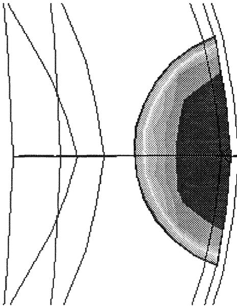
Fig. 3. Grout pressure distribution in the crack. Maximum pressure is 2.93 MPa, three injection points, time is 69.5 min.
