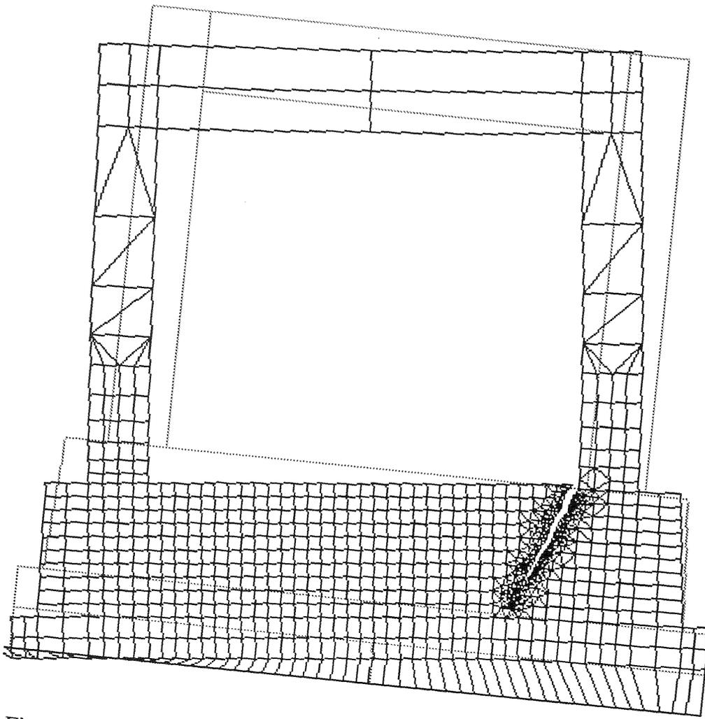
Fig. 8. Final deformed finite element mesh after fourteen 1 ft (0.30 m) increments of predicted cracking from Point A. Dead and live load, and 41 ft (12.5 m) of scour. Magnification factor is 25.
