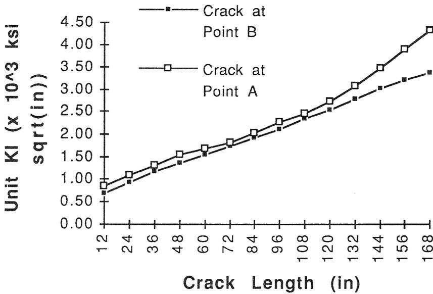
Fig. 11. Computed KI due to 1 kip (4.45 kN) post-tensioning force,
