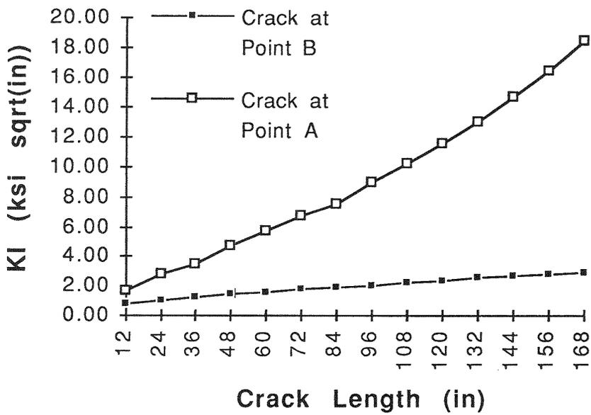
Fig. 10. Computed KI due to dead plus live load only.
