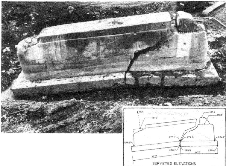
Fig. 6. Photograph of failed plinth. From Wiss87.
