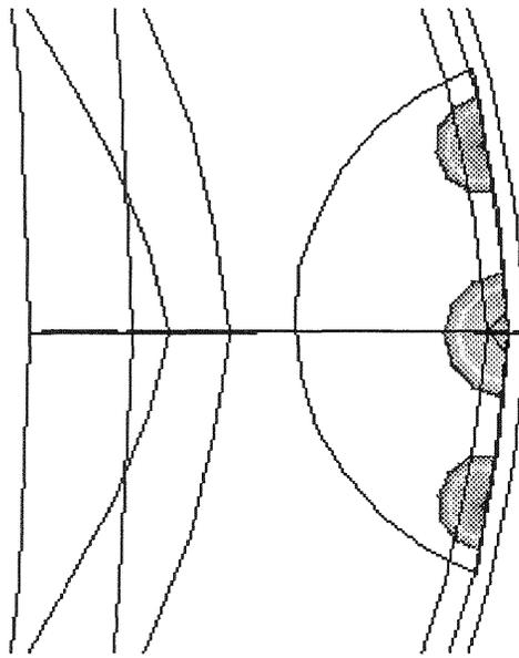
Fig. 2. Grout pressure distribution in the crack. Three injection points, time is 10 min.
