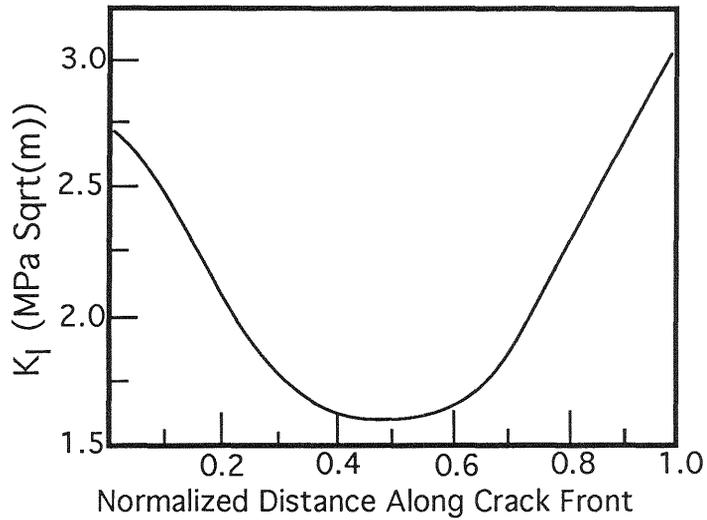
Fig. 4 Distribution of  $K_I$  along the crack front, three injection points,  $9 \times 10^{-4} \text{ m}^3/\text{s}$  total injection rate, 30 minutes injection time.
