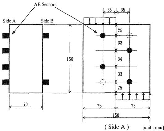
Fig. 2 Model test for shearing crack
