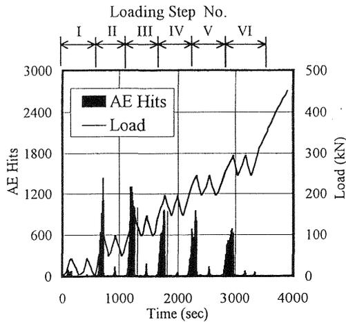
Fig. 12 Result of AE measurement for bending test
