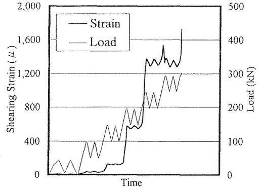
Fig. 15 Relationship between load and shearing strain
