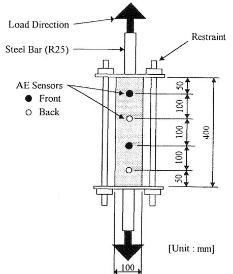
Fig. 4 Direct tension test
