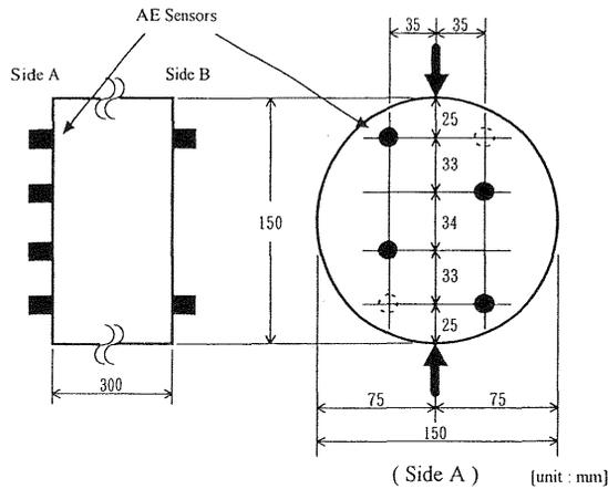
Fig. 1 Model test for bending crack
