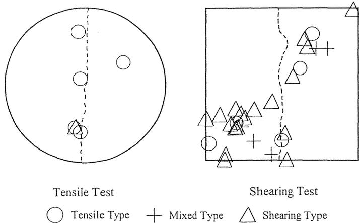
Fig. 8 Result of moment tensor analysis
