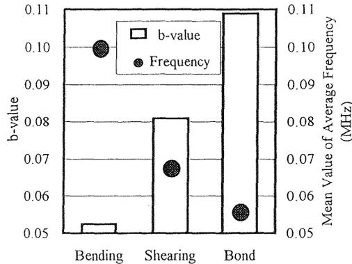
Fig. 11 Relationship between crack type and AE characteristics
