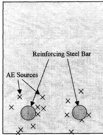
Fig. 14 Calculated AE sources around reinforcement
