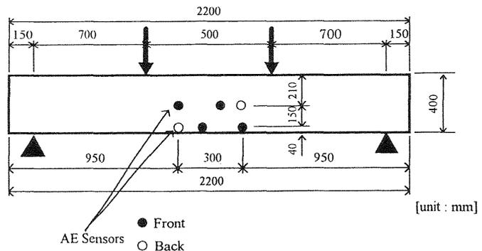
Fig. 5 Bending test on mock-up of RC beams
