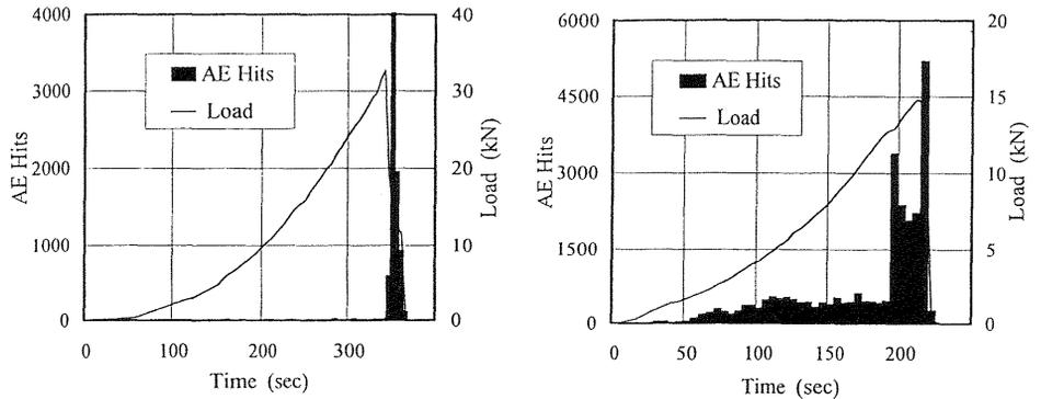
(a) Bending crack model test      (b) Shearing crack model test
