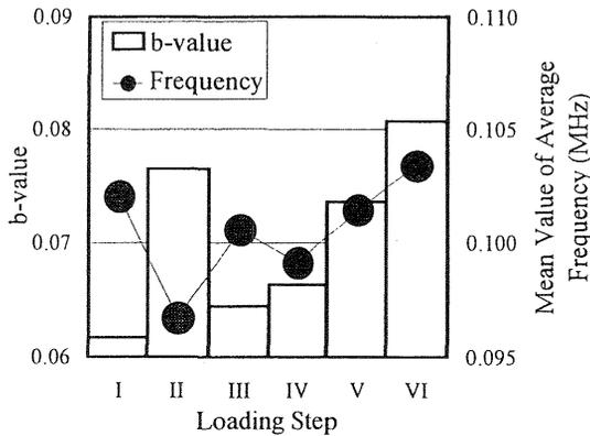
Fig. 13 Change in AE parameters during loading process
