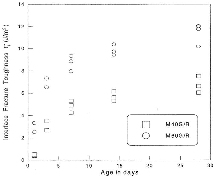
Fig. 3. Interface fracture toughness with mortar age
