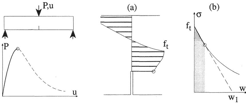
Fig. 2. Peak load situation for a notched beam. (a) Stress profile. (b) Softening function. The stress at the notch is marked with a circle.
