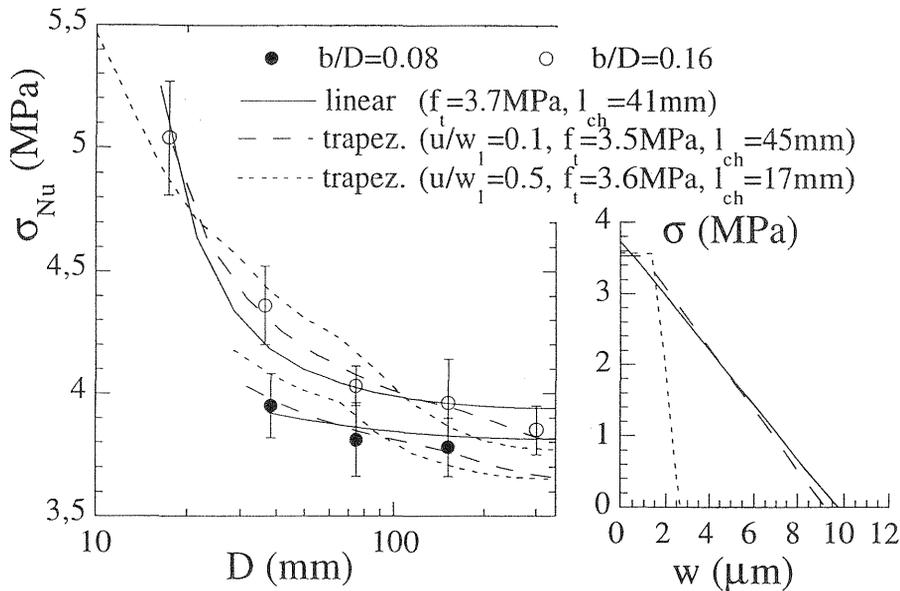
Fig.6. Size effect curves for Brazilian square specimens and best fit for linear and trapezoidal softening functions. Mean values (circled points) and 95% confidence interval are shown for each size.
