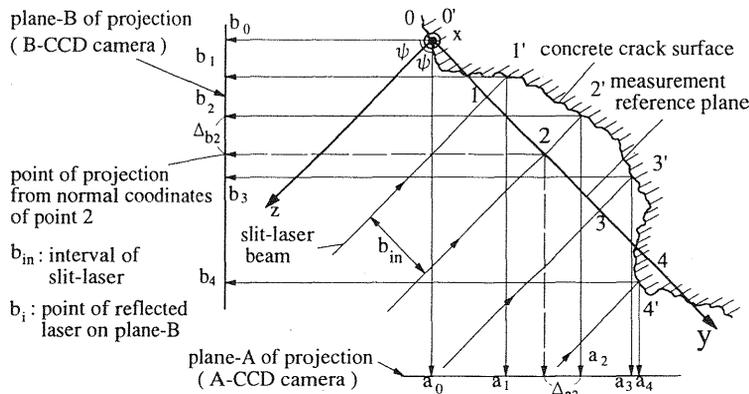
Fig. 3. Coordinate axes in the measurement system
