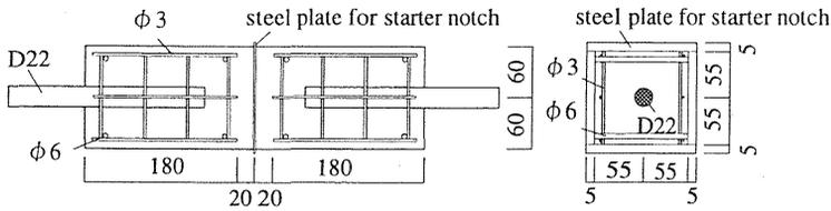
Fig. 7 Concrete specimen used in the tensile experiment
