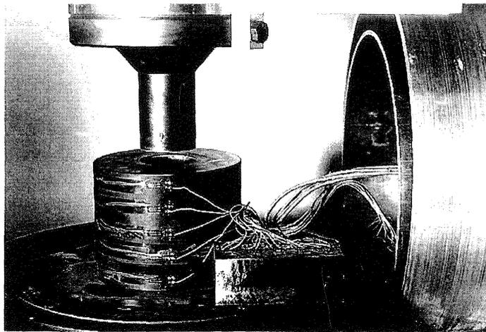
Fig. 2. Photograph of the uniaxial confined compression test.
