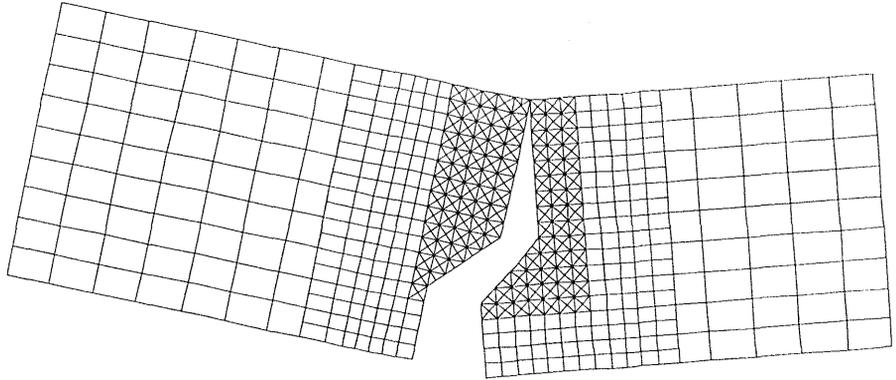
Figure 6. Deformed mesh obtained with aggregate interlock
