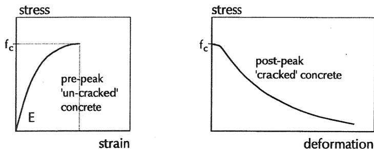
Fig 1. Pre-peak stress-strain curve (a) and post-peak stress-deformation curve (b) for concrete subjected to uniaxial compression, after Van Mier et al. (1997).
