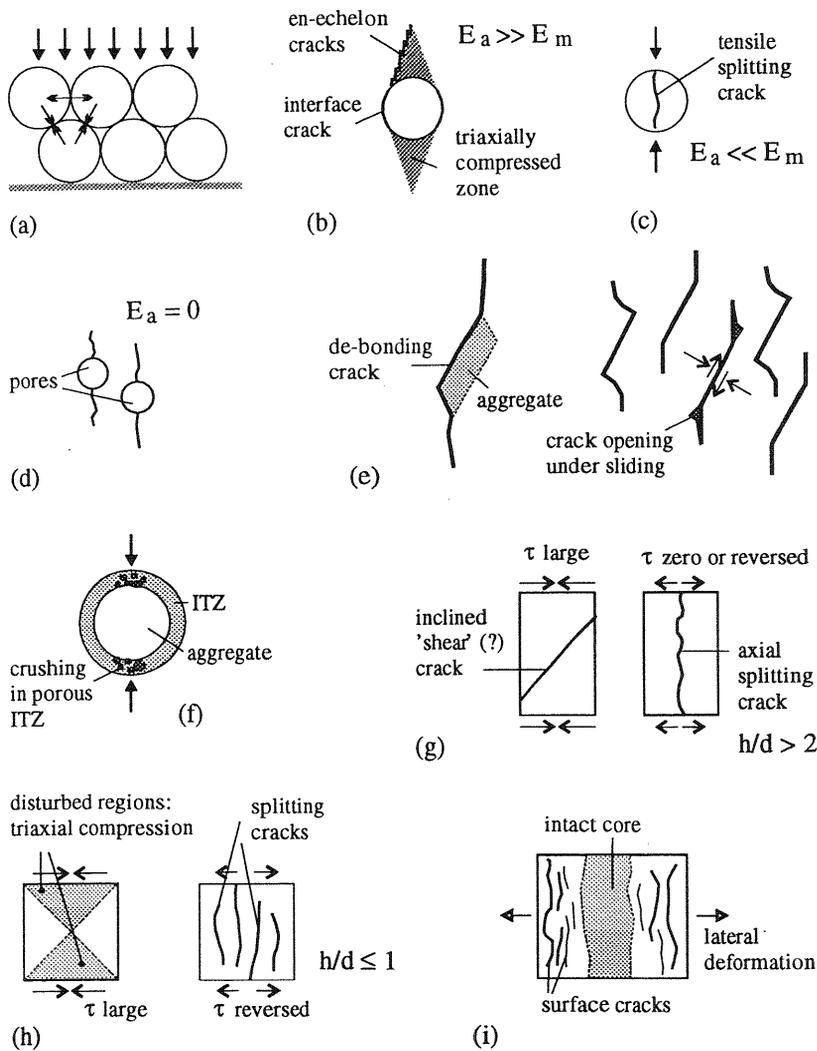
Fig. 3 Different mechanisms for the mechanical behaviour of concrete under uniaxial compression at the meso- and macro-level. The various mechanisms are explained in the text.
