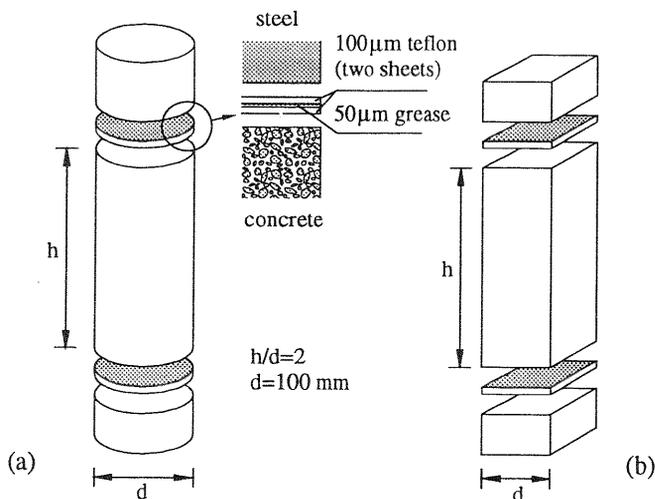
Figure 4 Standard test for determining the complete stress-strain diagram for concrete under uniaxial compression, after Van Mier (1997b).
