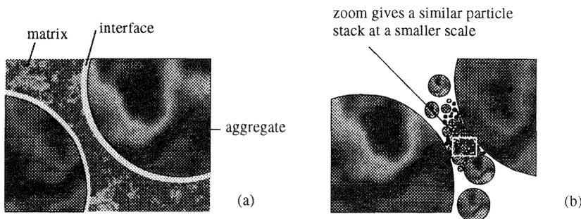
Fig. 2 Concrete regarded as particles 'swimming' in a matrix of cement (a), or as a stack of particles with different size (b), after Van Mier (1997a).
