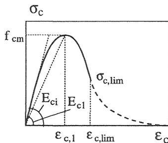
Fig. 5 Stress-strain diagram for uniaxial compression according to the CEB-FIP Model Code 1990.
