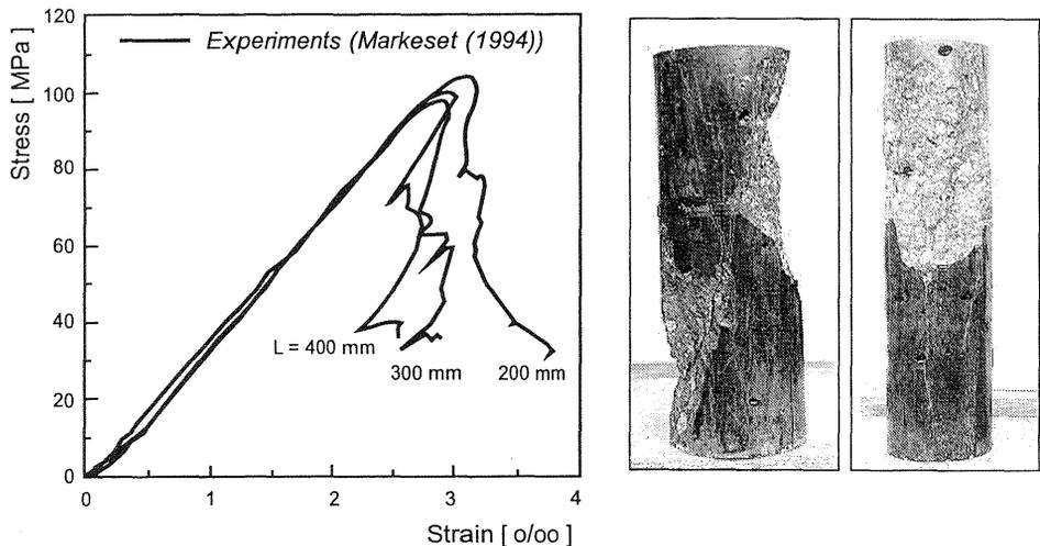
Fig. 2. Influence of specimen length on the complete stress-strain curve, and formation of shear band and damage zone, Markeset (1994). Cylinder diameter is 100 mm
