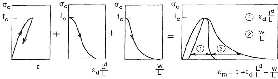
Fig. 7. Composition of the complete stress-strain curve, Markeset (1993)
