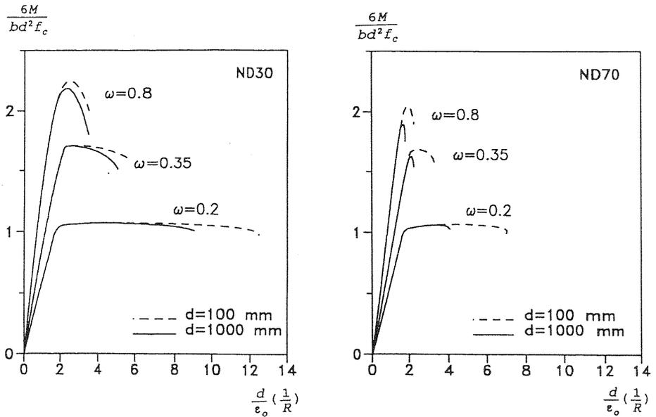
Fig. 11. Calculated moment-curvature diagram (dimensionless numbers) for effective beam depth  $d=100$  and  $1000$  mm, Markeset (1993)
