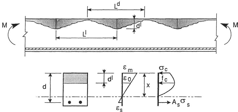
Fig. 8. Damage localizations in a bent beam, Markeset (1993)
