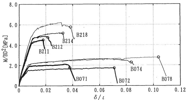
Fig. 3. Normalized bending moment-displacement curves, Adachi et al. (1995)
