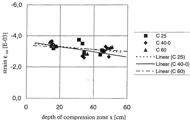
Fig. 4. Ultimate concrete strain,  $\epsilon_{cu}$ , versus depth of the compression zone, Meyer (1997)
