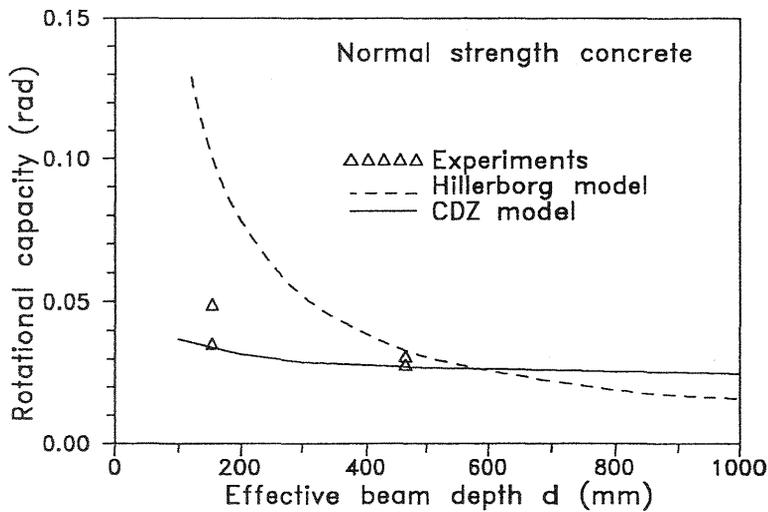
Fig. 10. Size effect on rotational capacity, Markeset (1993)
