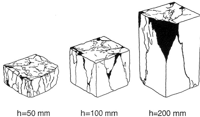
Fig. 1. Crack patterns of normal strength concrete prisms, van Vliet and Mier (1996)
