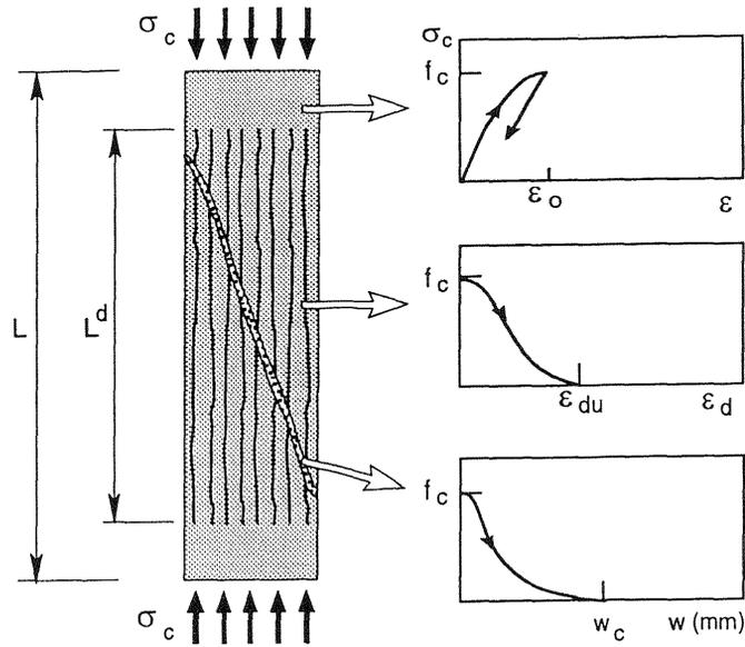
Fig. 6. Illustration of the CDZ model on a specimen loaded in uniaxial compression, Markeset (1993)
