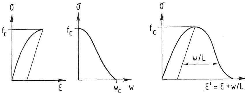
Fig. 5. Stress-deformation curve for the localized zone as a part of the complete compressive stress-strain curve for a gauge length  $L$ , Hillerborg (1988)
