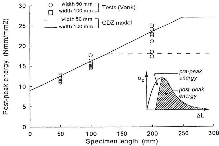
Fig. 9. Post-peak energy for different specimen geometries, Markeset and Hillerborg (1995)
