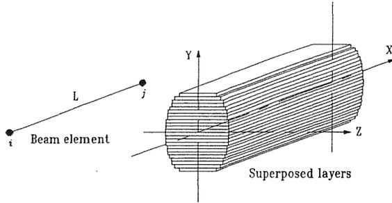
Fig. 1. EFICOS program: Superposed layer beam elements
