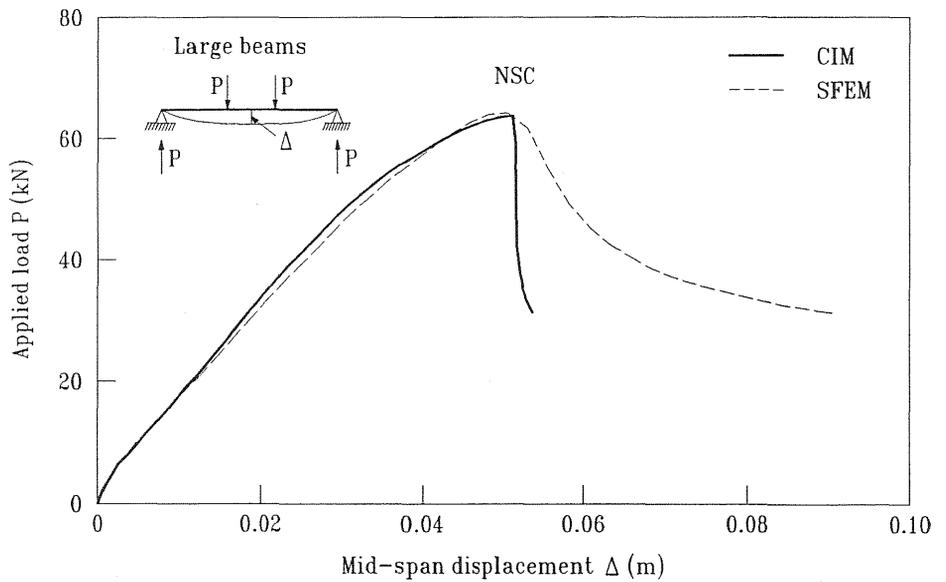
Fig. 6. Predicted mid-span displacement-applied load, large beams
