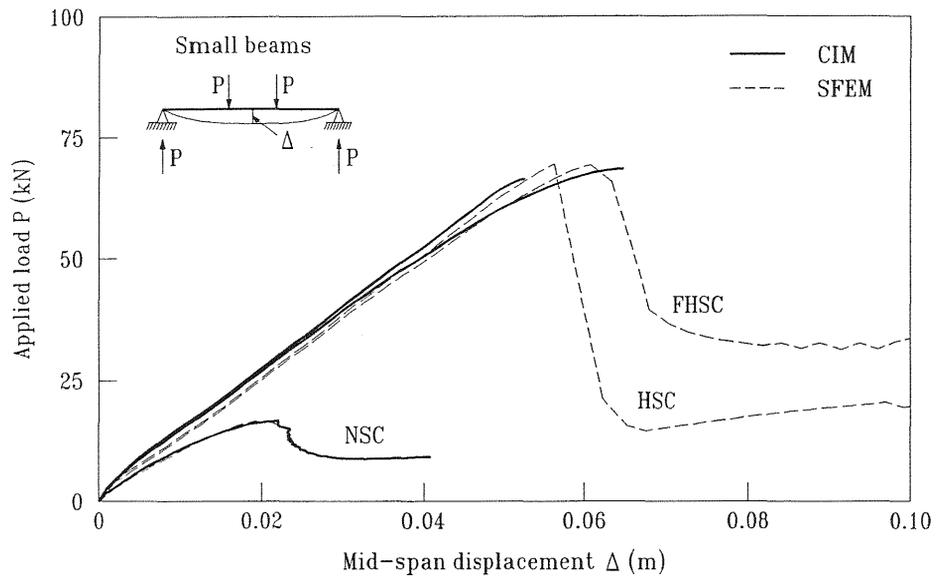
Fig. 5. Predicted mid-span displacement-applied load, small beams
