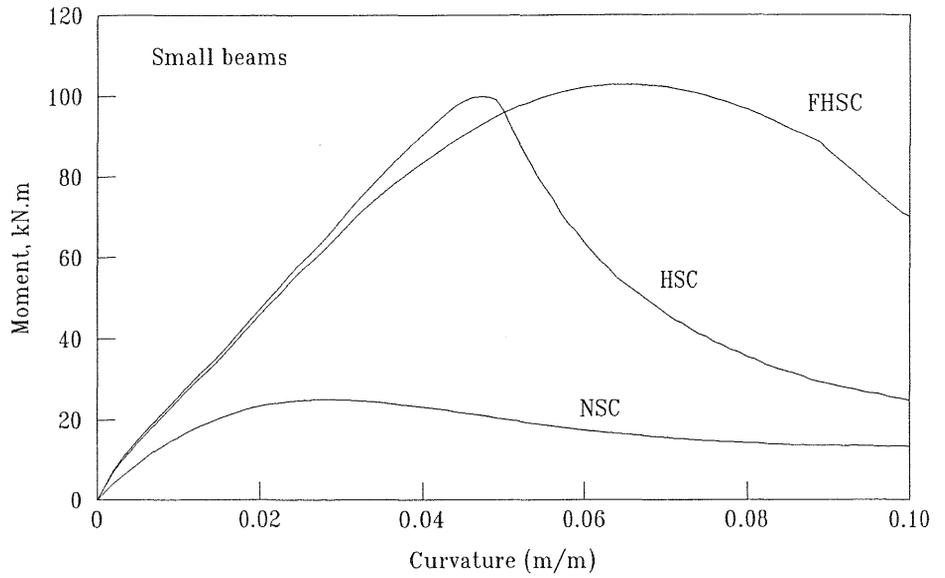
Fig. 3. Predicted curvature-moment response for small beams
