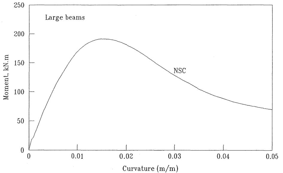
Fig. 4. Predicted curvature-moment response for large beams
