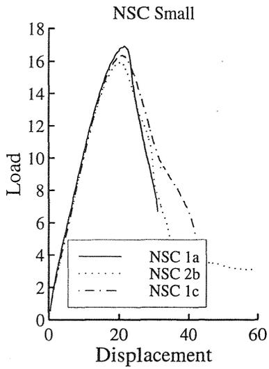
Fig. 2. Load displacement curves for NSC for the small beams.
