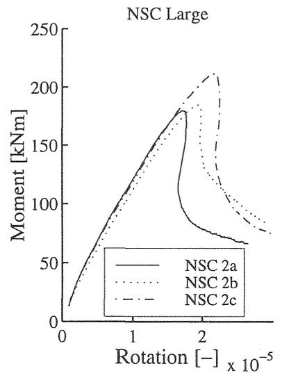
Fig. 9. Moment rotation curves for NSC for the large beams.
