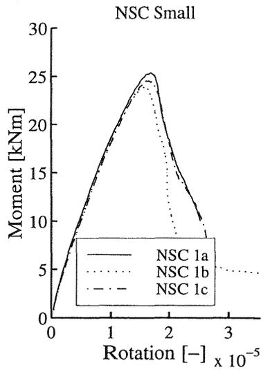
Fig. 3. Moment rotation curves for NSC for the small beams.
