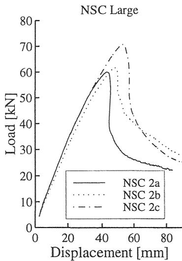
Fig. 8. Load displacement curves for NSC for the large beams.
