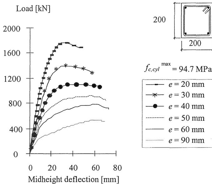
Fig. 3 Load-deflection curve of a 4 m high-strength concrete column subjected to different initial load eccentricities.
