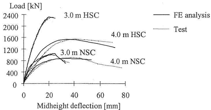
Fig. 1 Comparison between the results from the tests and those of the FE analysis
