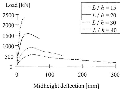
Fig. 5 Effect of slenderness on high-strength concrete columns subjected to an eccentricity of 20 mm.
