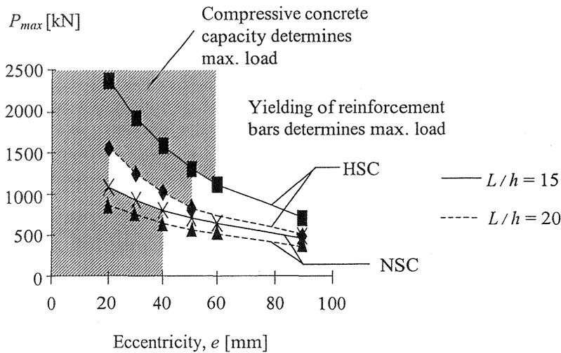
Fig. 4 The effect of eccentricity on the maximum load of different slenderness ratios and concrete strengths
