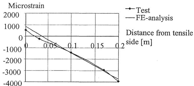
Fig. 2 Strain distribution at maximum load for a 3m high-strength concrete column with stirrup spacing 130 mm
