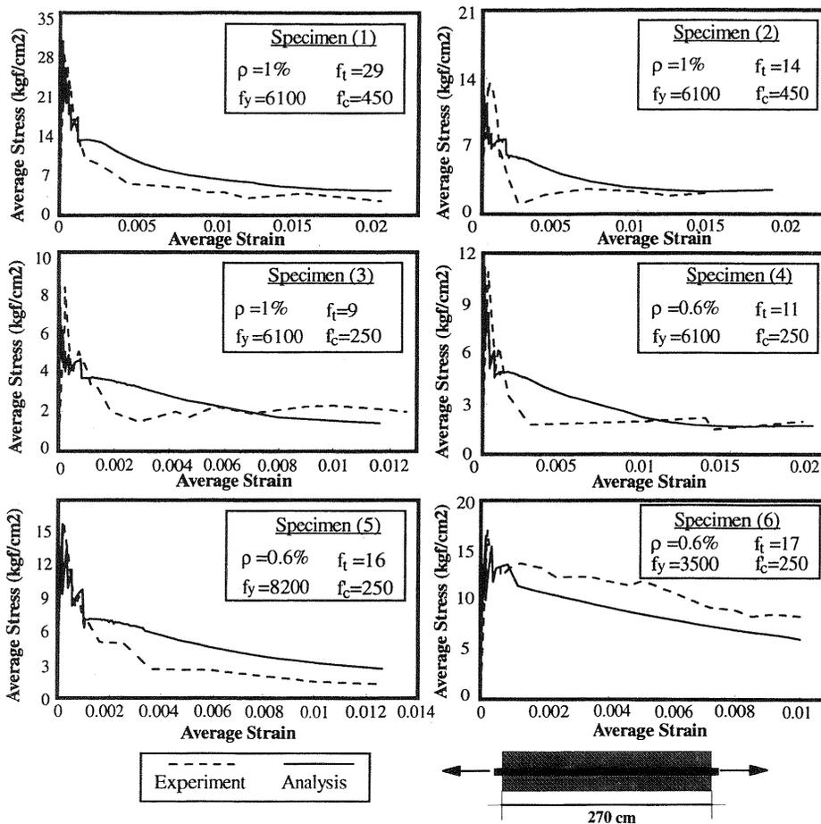
Fig.5. Average response of concrete: A comparison with the experimental work of Shima et al. (1987)
