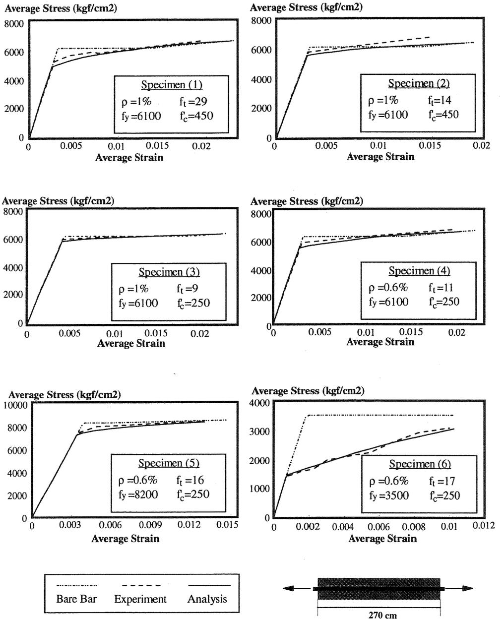
Fig.6. Average response of reinforcement: A comparison with the experimental work of Shima et al. (1987)
