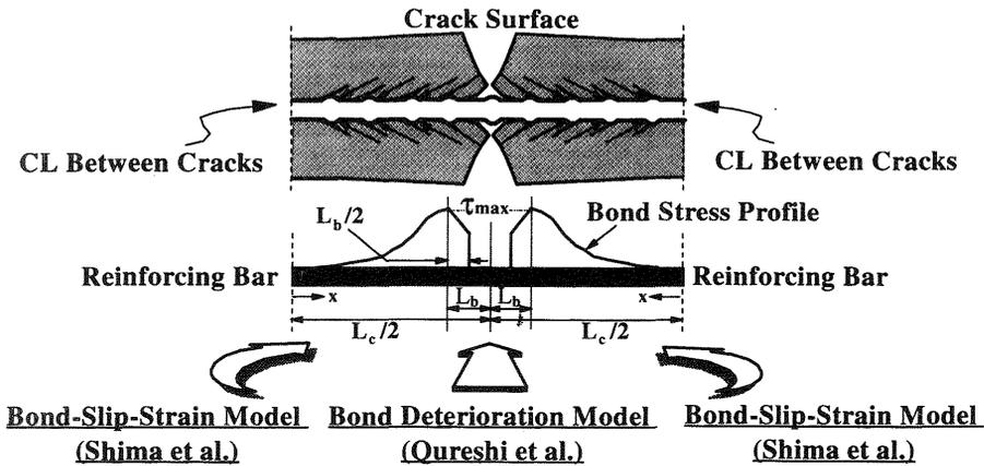
Fig.1 Bond deterioration zone by Qureshi et al. (1993)
