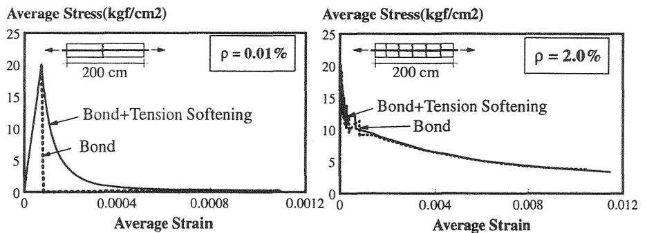
Fig.3. Tension softening effect on tension stiffness of RC
