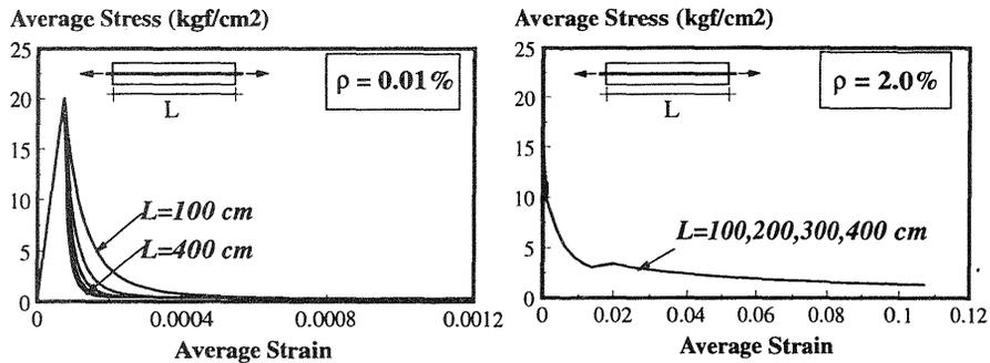
Fig.4. Size effect on average response of concrete
