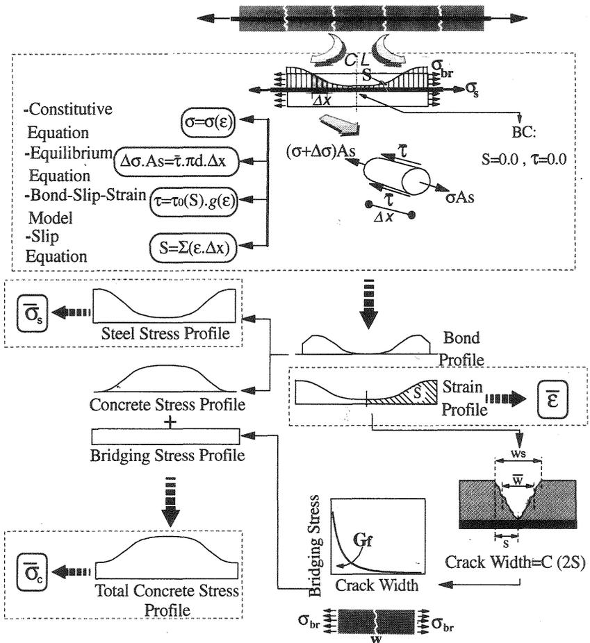
Fig.2. Scheme of solving bond governing equations with finite discretization
