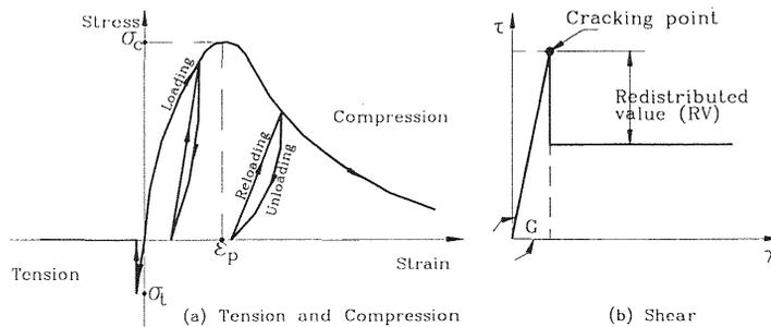
Fig. 3 Tension, compression and shear models for concrete
