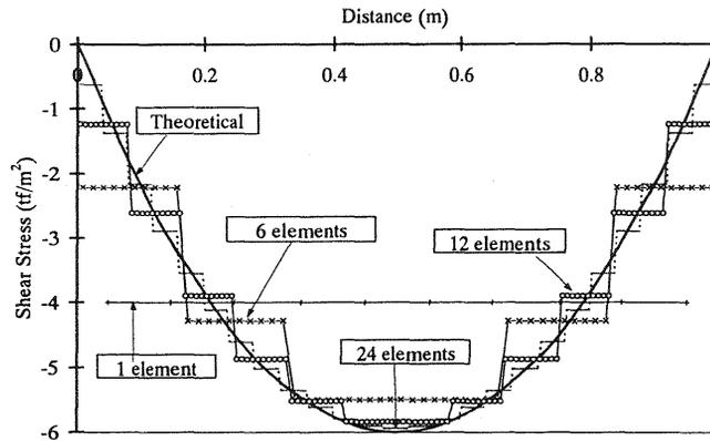
Fig. 7 Shear stress distribution at the column base
