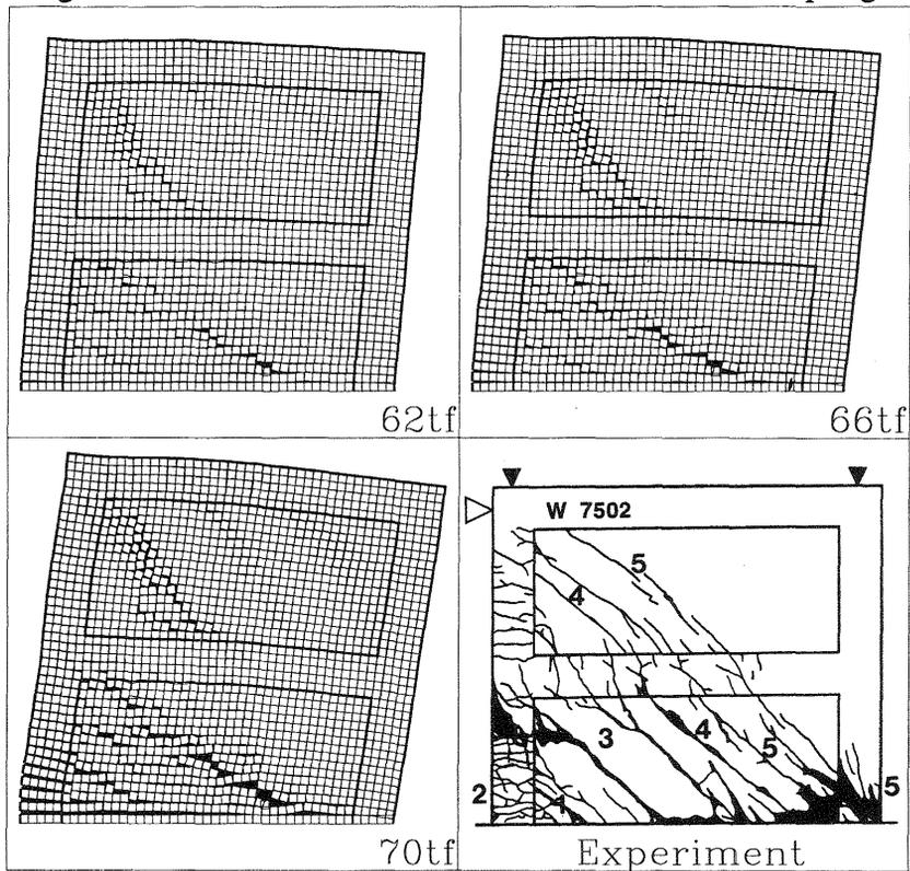
Fig. 10 Deformed shape and crack locations of the 2-storied RC wall structure (in case of 500 increments with 10 springs between each two adjacent faces, Simulation Scale Factor=30)
