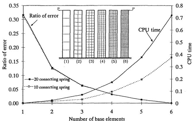
Fig. 5 Relation between the number of base elements, ratio of error and CPU time
