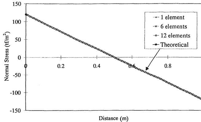
Fig. 6 Normal stress distribution at the column base
