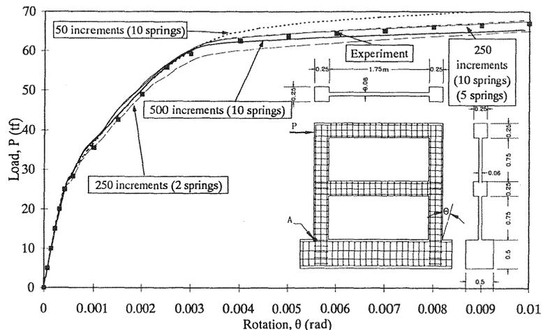
Fig. 8 Relation between load and wall rotation for 2-storied RC wall
