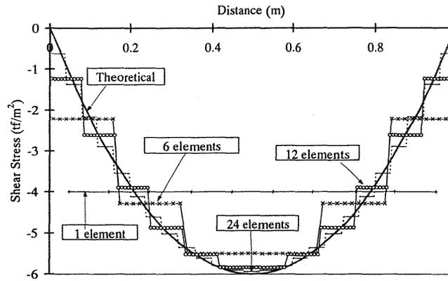
Fig. 7 Shear stress distribution at the column base
