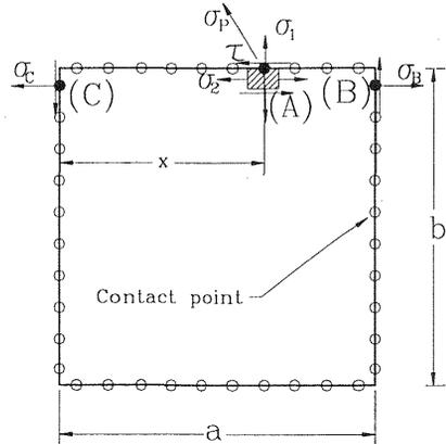
Fig. 4 Principal Stress determination
