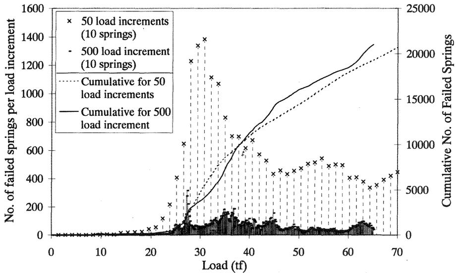
Fig. 9 Relation between load and the number of failed springs
