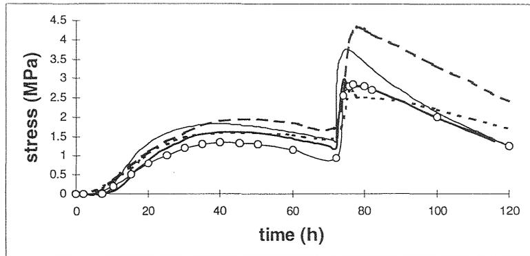
Fig. 1. Stresses calculated by five different computer programs
