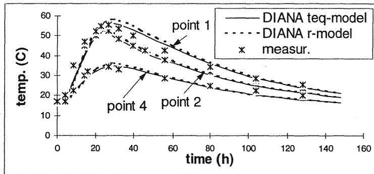
Fig. 8 Temperature development in the wall, calculations results based on equiv. age and degree of hydration compared to measurements
