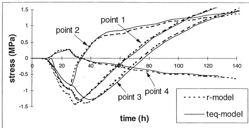
Fig. 9 Stress development in the wall, calculations results based on equivalent age and degree of hydration
