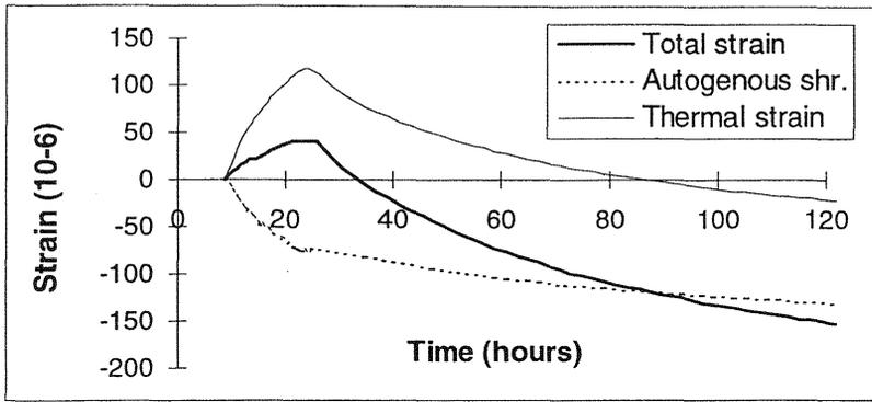
Fig. 5 Stress independent strain determined from the shrinkage rig, (concrete 1) under realistic temperature development
