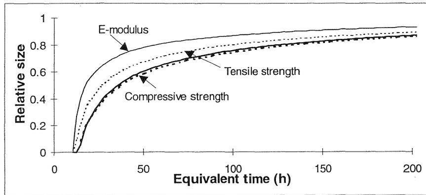
Fig. 4. Relative development of different model parameters
