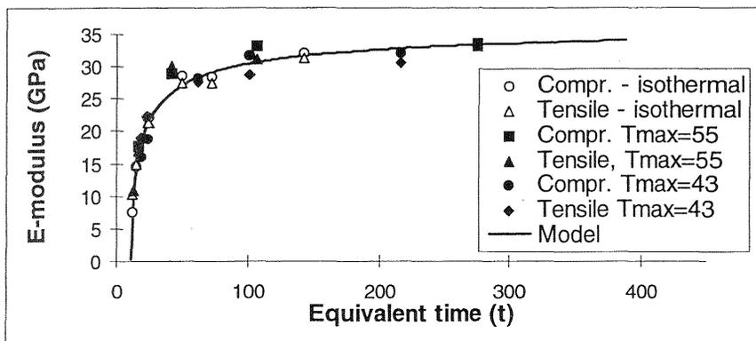
Fig. 2. E-modulus versus equivalent age
