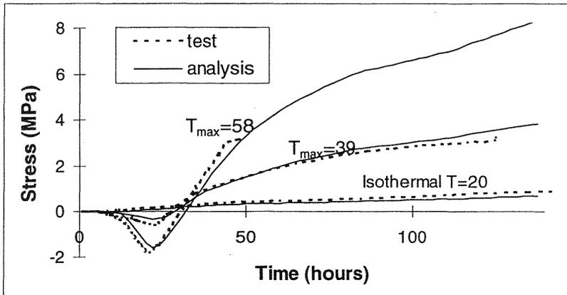
Fig. 6 Experimental and calculated results from the temperature-stress machine, (a) concrete 1, (b) concrete 2
