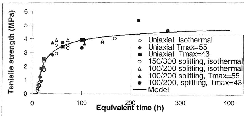
Fig. 3. Tensile strength versus equivalent age
