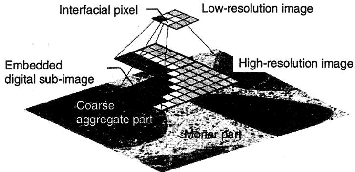
Fig. 4. Tree-structured hierarchical digital image
