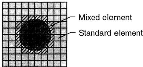
Fig. 8.1. Mixed element mesh
