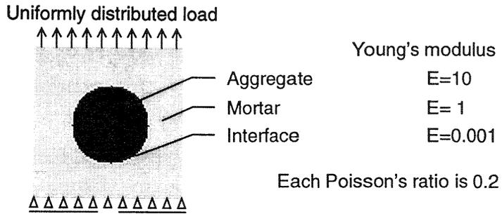
Fig. 7. Simple 80<sup>2</sup> pixels model
