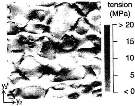
Fig. 3. Maximum principal stress in the center of  $y_2$ - $y_3$  section
