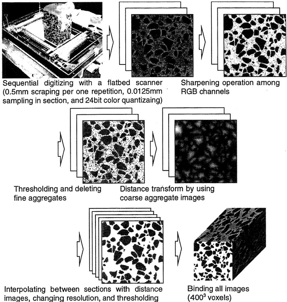
Fig. 1. Image digitizing and processing procedure
