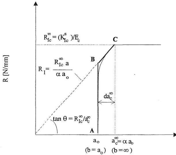
Fig. 2. A simplified  $R$ -curve approach for brittle cement-based matrices
