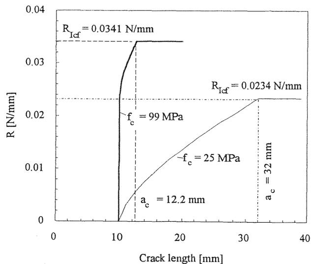
Fig. 1. Characteristic  $R$ -curves for normal and high strength concrete
