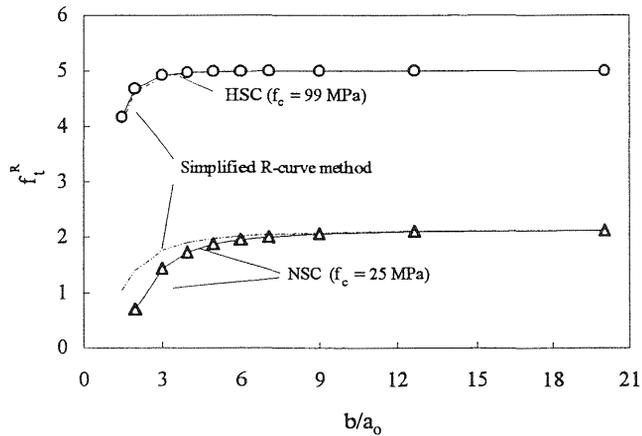
Fig. 5.  $f_t^R$  for specimens of different width and strength
