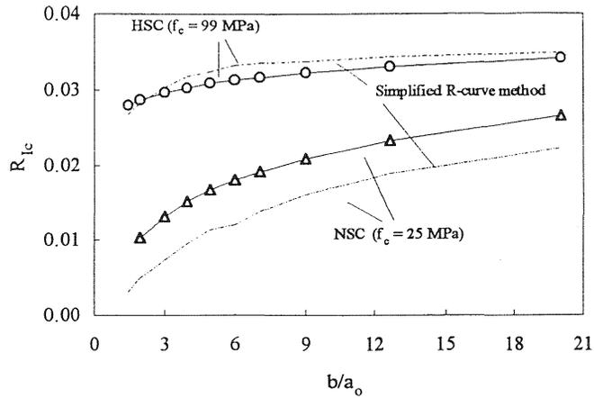
Fig. 4.  $R_{Ic}$  for specimens of different width and strength
