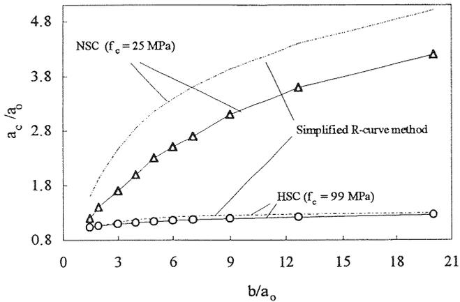
Fig. 3.  $a_c$  for specimens of different width and strength
