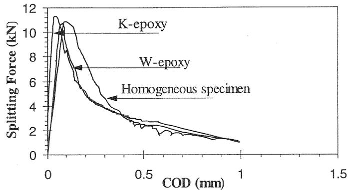
Fig. 8. Response of repair material at room temperature for dry condition
