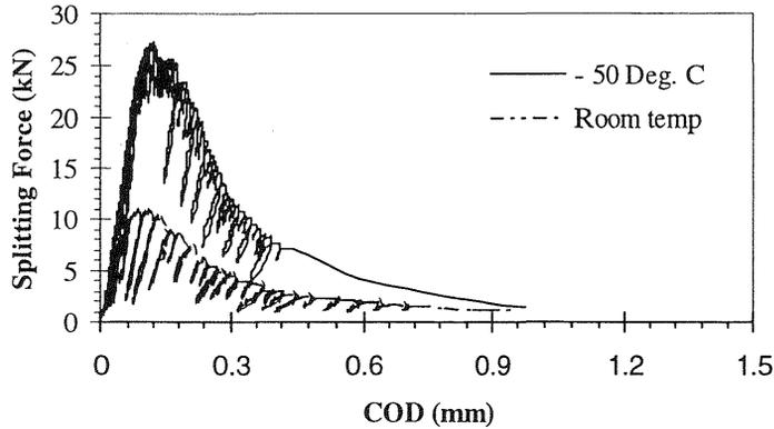
Fig. 3. Response of specimen cast in two blocks at low and room temperature
