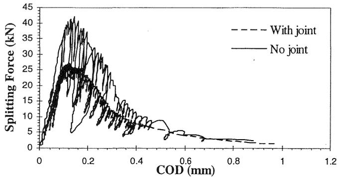
Fig. 4. Effect of simulated joint on the material response at low temperature
