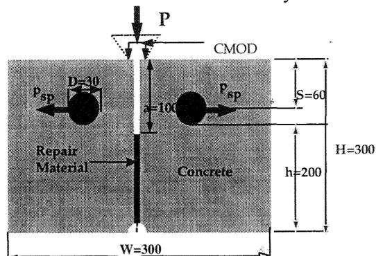
Fig. 1. Specimen geometry (mm)
