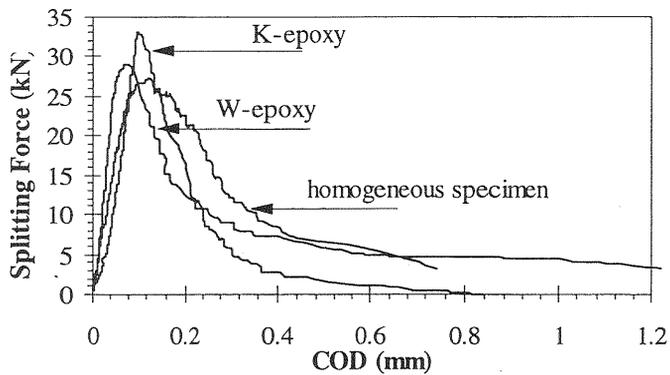
Fig. 6. Response of repair material at low temperature for dry condition
