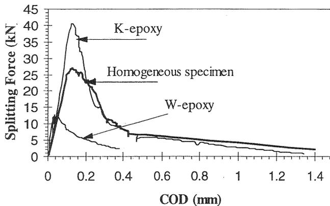
Fig. 7. Response of repair material at low temperature for wet condition
