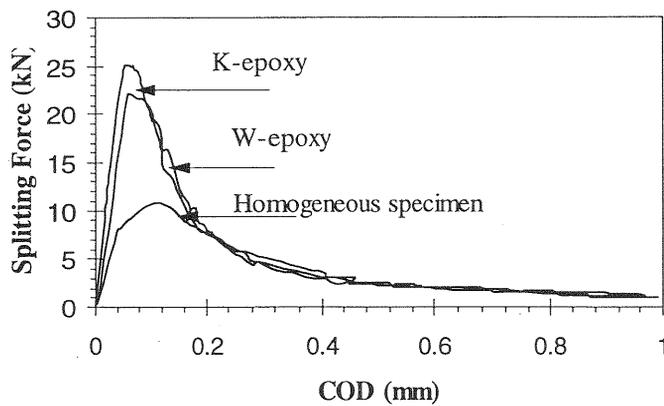
Fig. 9. Response of repair material at room temperature for dry condition
