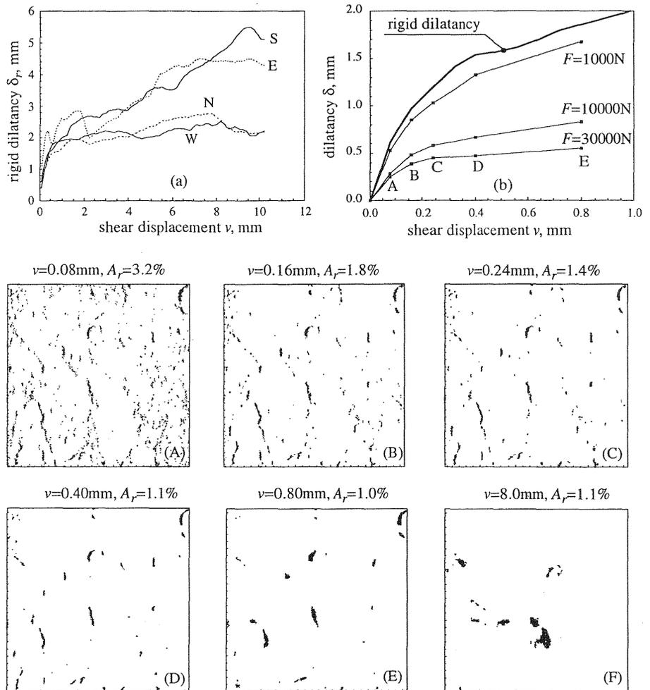
Fig. 5. Rigid dilatancy curves (a), elastic dilatancy curves (West direction) (b), contact domains corresponding to points A-E on the  $F=30000\text{N}$  curve.
