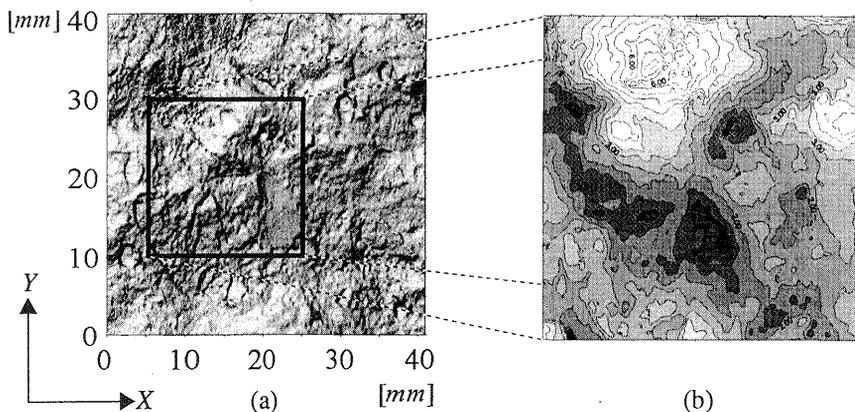
Fig. 1. Shaded relief of the fracture surface (a), and *delta-surface* from the  $2\times 2\text{ cm}^2$  central portion shifted 8mm in the West (see Fig. 2) direction (b).
