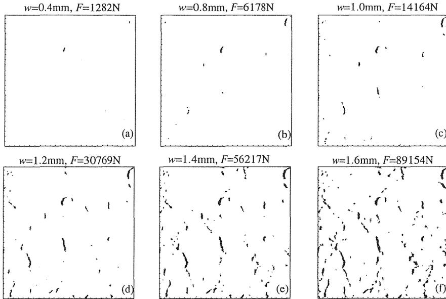
Fig. 4. Evolution of the contact domain during crack closure for  $v=0.4\text{mm}$  (see the related points in Fig. 3a).
