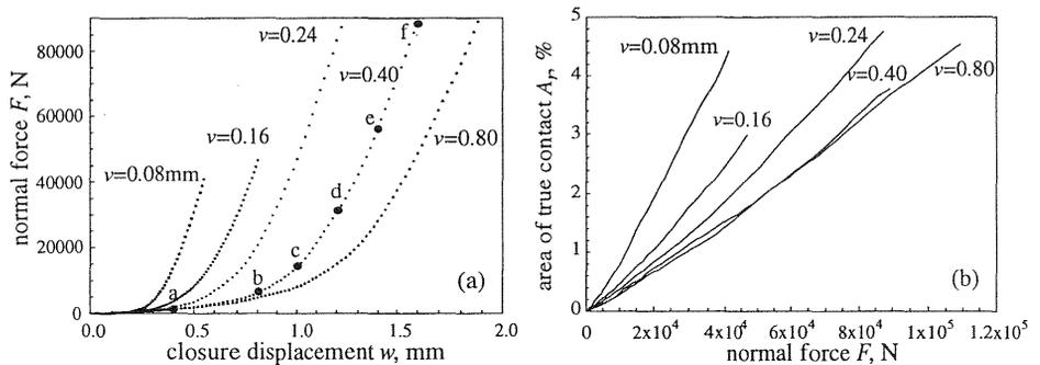
Fig. 3. Crack closure laws (a), and real contact area vs. applied force (b).
