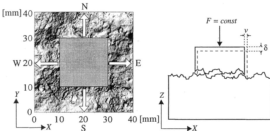
Fig. 2. Scheme of the simulation: dilatancy ( $\delta$ ) and shear displacement ( $v$ ).
