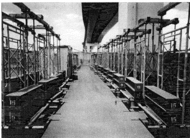
Fig. 3 View of creep rupture test
