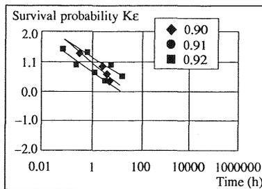
Fig. 4. Survival probability of 12.5 mm dia. CFRP
