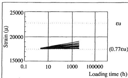
Fig. 13. Creep strain of AFRP case 1
