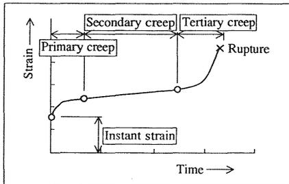
Fig. 11. Creep strain model diagram
