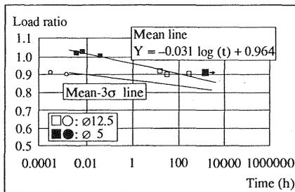
Fig. 9. Load ratio and creep fracture time of CFRP
