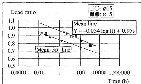
Fig. 10. Load ratio and creep fracture time of AFRP
