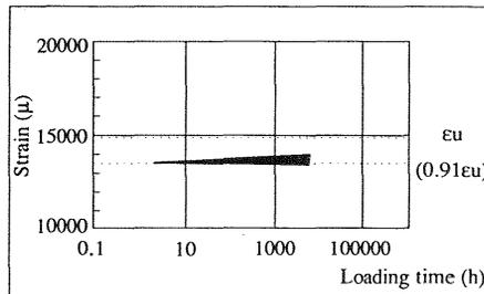
Fig. 12. Creep strain of CFRP
