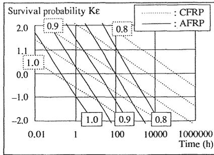
Fig. 8. Schematic diagram of survival probabilities
