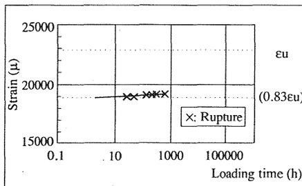
Fig. 14. Creep strain of AFRP case 2
