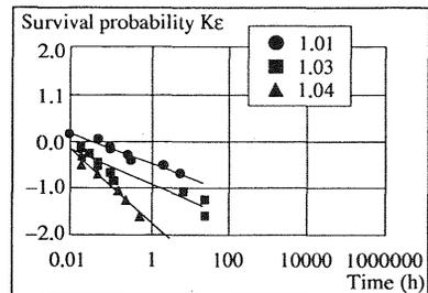
Fig. 5. Survival probability of 5 mm dia. CFRP
