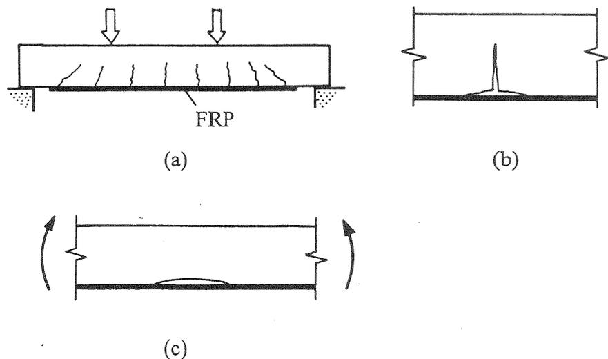
Fig. 1. (a) Flexural strengthening of RC beam; (b) FRP-concrete interface crack due to flexural cracking; and (c) interface crack due to unevenness of the concrete surface.
