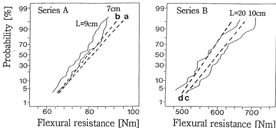
Fig. 6. Comparison between theoretical values obtained from the series linking model and measured values
