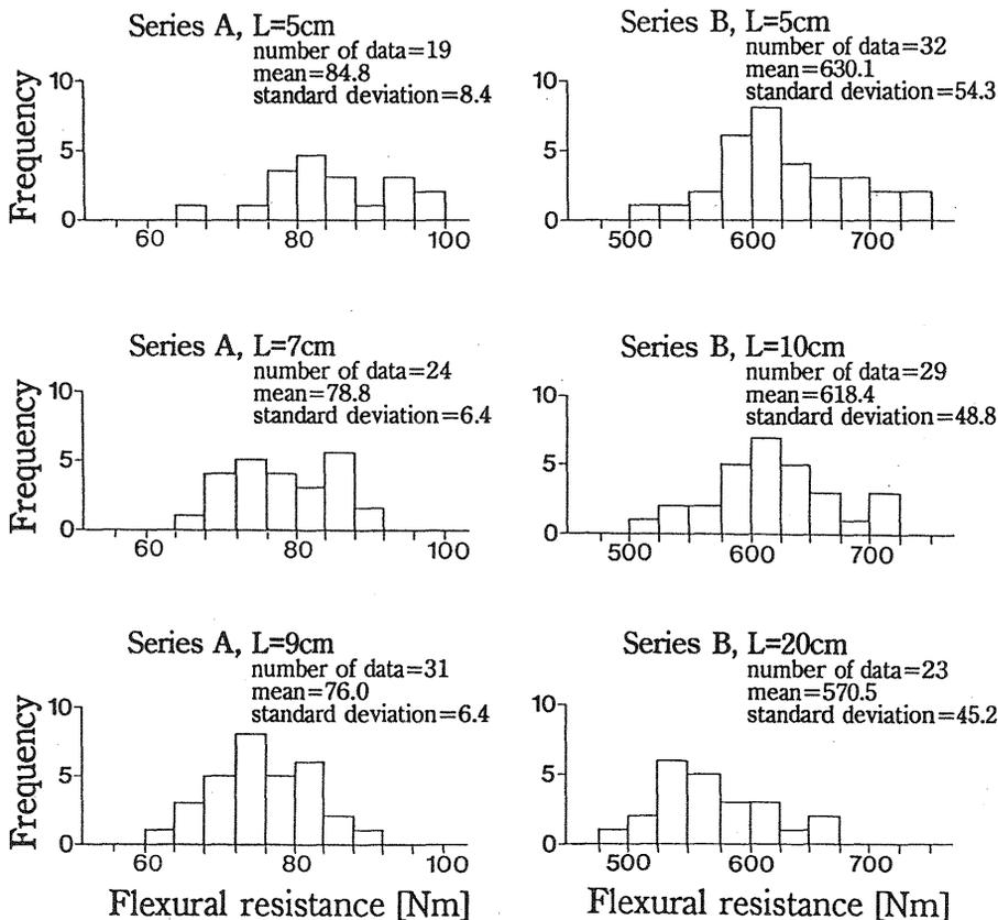
Fig. 2. Flexural resistance distribution
