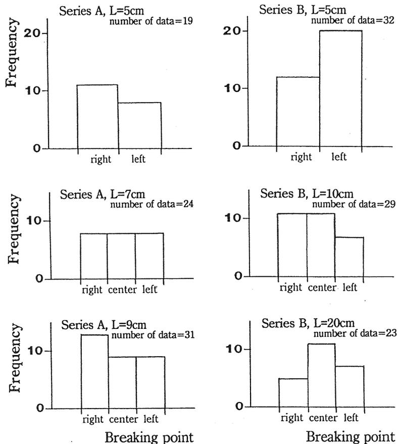
Fig. 3. Distribution of breaking points in test specimens
