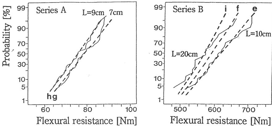
Fig. 7. Comparison between theoretical values obtained from the proposed model and measured values
