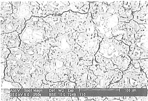
Figure 5. Micrograph of HCP, BSE imaging, 90 days.
