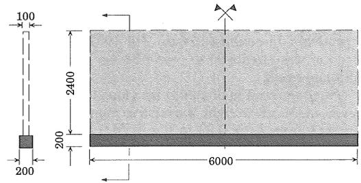
Figure 2: Numerical example: Geometry of the concrete wall (van Zijl 1999) (Dimensions in [mm]) restrained at the base by a non-shrinking foundation, is described in this section. A similar numerical example has been investigated by (van Zijl et al. 1998; van Zijl 1999), who analysed masonry walls subjected to restrained shrinkage.
