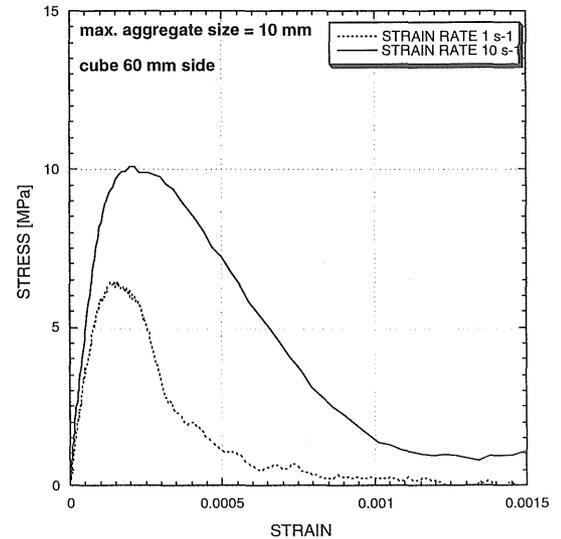
Figure 4. Stress vs. strain curves for two strain-rates
