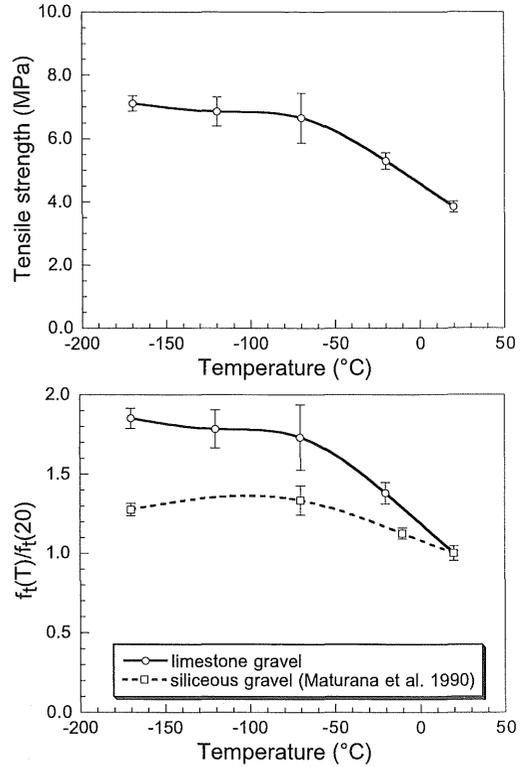
Figure 2. Effect of low temperatures on the splitting tensile strength: absolute values (top), and comparison of values relative to that at 20 °C with the results of Maturana et al. (bottom).
