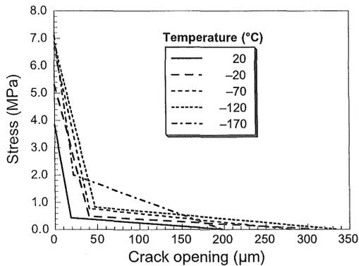
Figure 4. Softening curve of concrete at various temperatures.
