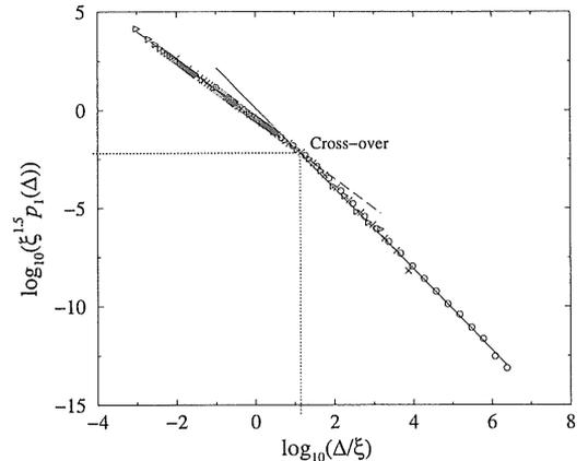
Figure 2: The avalanche distribution for zip model with a constant beam shape. The active area size  $\xi$  are 100 ( $\circ$ ), 1000 ( $\times$ ) and 10000 ( $\triangleright$ ). The dashed line is a guide line with a slope of -1.5. The continuous lines is a guide line with a slope of -2.05.
