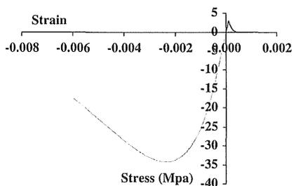
Figure 2: uniaxial response of the model by Mazars (1984).
