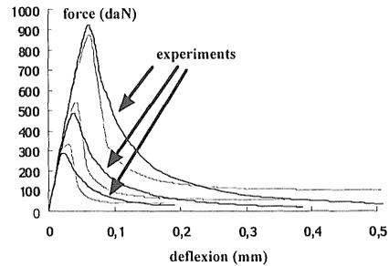
Figure 10: Fit of the non local model with the size effect test data (after Le Bellégo et al. 2000).
