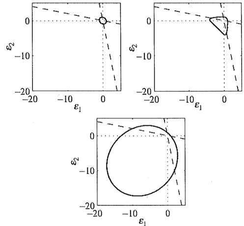
Figure 1: Contour plots for  $\tilde{\varepsilon}$  for the elastic stored energy (top left), Mazars definition (top right), and the modified von Mises expression (bottom), after Peerlings et al. (1998).
