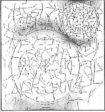
Figure 11: Fictitious cracks in a section of the model subjected to direct tension of specimen 3.
