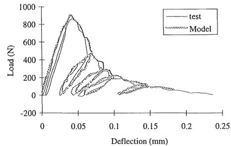
Figure 6. Experimental and predicted results for cyclic loops.
