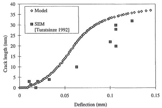
Figure 5. Observed and predicted crack length evolution.
