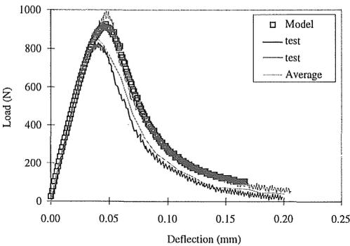
Figure 4. Measured and predicted load-deflection curves.
