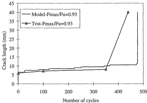
Figure 8. Crack length versus number of cycles. Comparison between the model and the experimental data : Example2.
