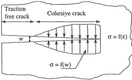
Figure 1. Sketch of the cohesive crack model.
