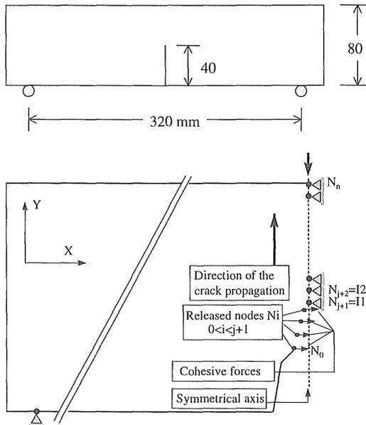
Figure 2. Modeling the beam. Boundary conditions.
