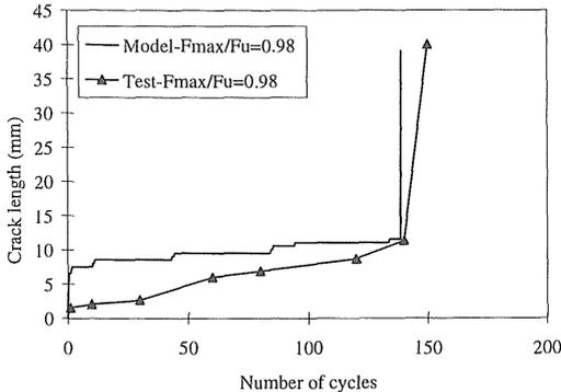
Figure 7. Crack length versus number of cycles. Comparison between the model and the experimental data : Example1.
