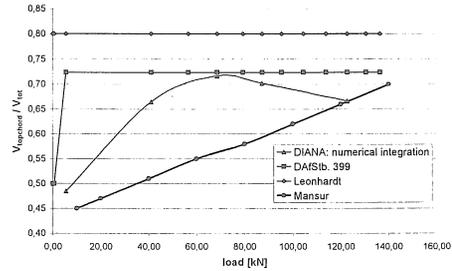
Figure 7. Shear force distribution on the chord of beam R3
