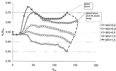
Figure 8. Shear force distribution for  $\alpha_t=0,19$
