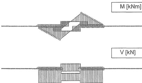
Figure 3b: Internal forces M and V due to  $P_Q$
