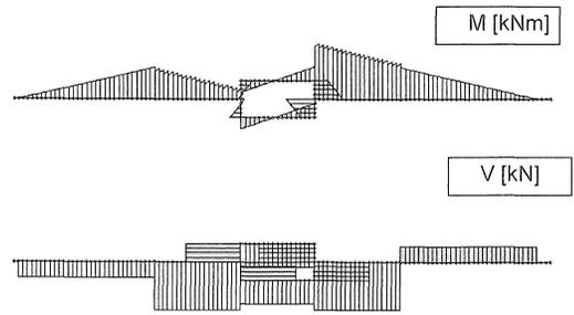
Figure 3c: Internal forces M and V due to  $P_M$  and  $P_Q$
