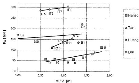
Figure 1. Influence of the opening's location on the ultimate load
