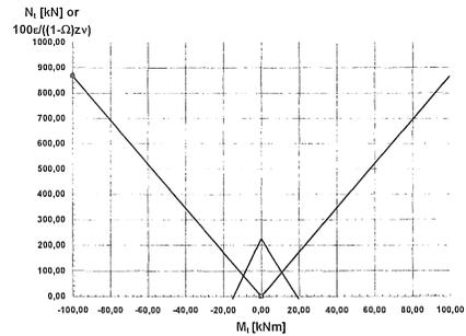
Figure 15. Outline of an M-N-interaction diagram for the determination of the first plastic hinge
