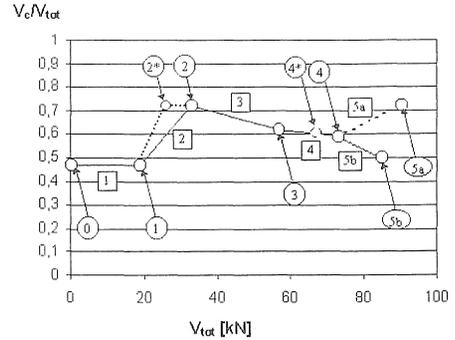
Figure 14. Outline of the evaluation of the shear force distribution (Kripos 2001)
