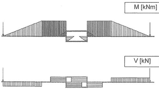
Figure 3a: Internal forces M and V due to  $P_M$
