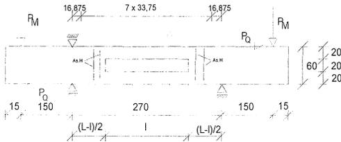
Figure 2: Testing scheme
