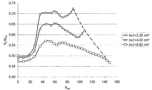
Figure 9. Shear force distribution for  $M/V=0,5$  m
