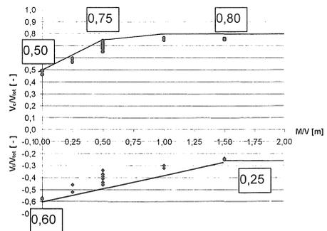
Figure 13. Estimating the shear force distribution for rectangular beams with  $l_1/l_c=1,0$  (Krips 2001)
