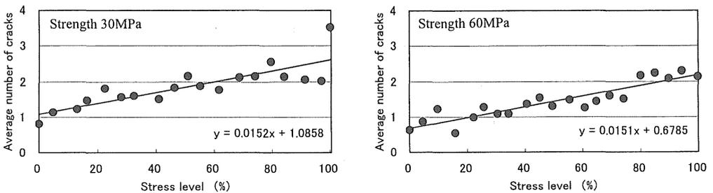
Figure 8. Correlation between Poisson parameters (average crack number,  $m$ ) and stress levels.
