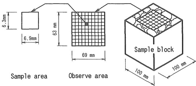
Figure 1. Sample areas used for microscopy.
