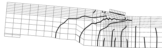
Figure 12. Deformed FE mesh with embedded cracks
