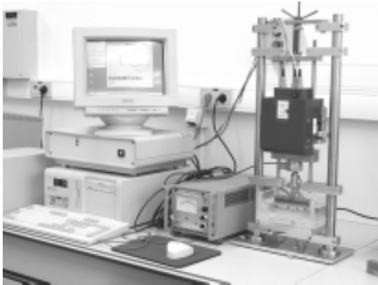
Figure 1. Developed mini test bank device for implementation into the X-ray chamber.
